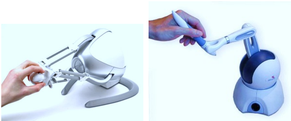
Figure 2.10: Two commercially available haptic devices: Novint Falcon (left) and Geomagic Touch.
