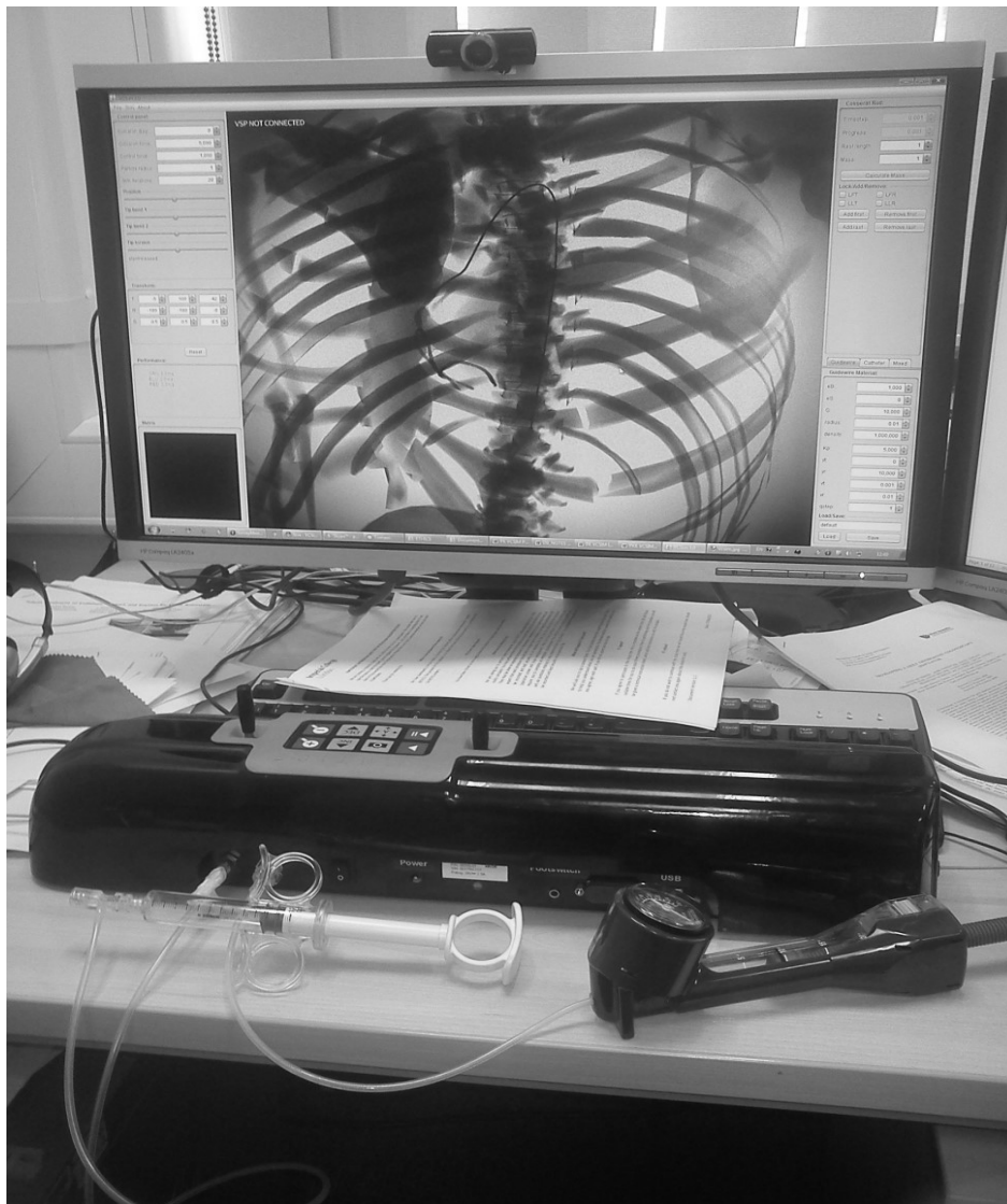
Figure 0.3: A complete experimental set-up. On the desk, the haptic device (black box) with a syringe and a balloon inflation device connected. On the computer screen, a running simulation software.
