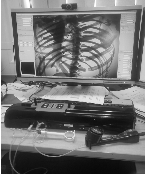
Figure 0.1: A complete experimental set-up. On the desk, the haptic device (black box) with a syringe and a balloon inflation device connected. On the computer screen, a running simulation software.
