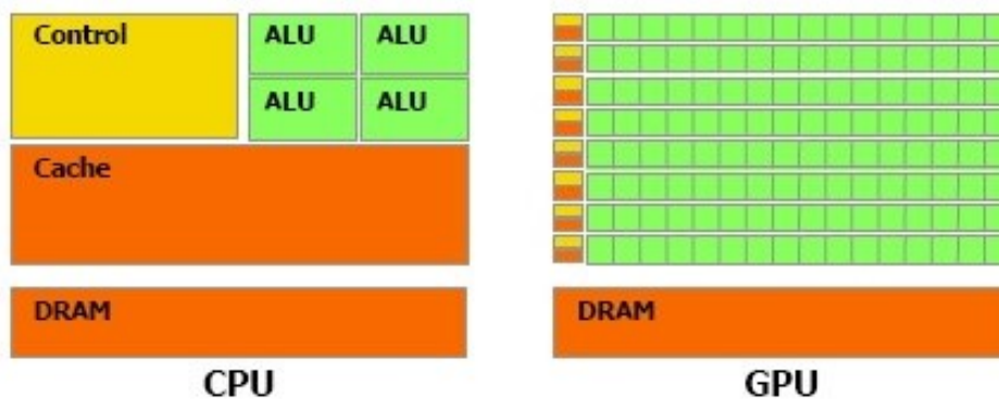
Figure 6.1: CPU vs GPU architecture comparison. (NVidia, 2014)
