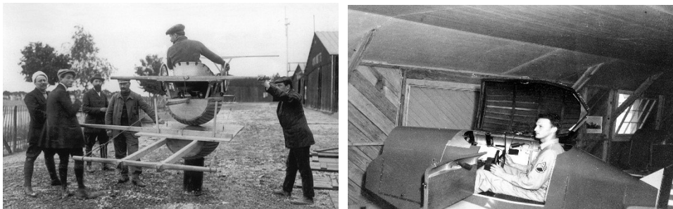
Figure 2.1: Left: The Antoinette training rig considered as the first flight simulator (1909). Right: The Link Trainer, the first widely adapted flight simulator (1930s-1950s).
