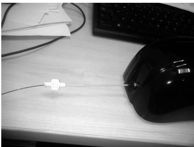
Figure 0.2: A zoom in at the real instruments (a guidewire inside a catheter) inserted into the haptic device (VSP).
