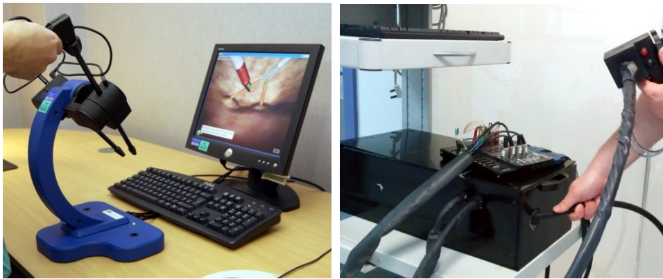
Figure 1.4: Two examples of VR simulators: On the left: LapSim simulator ( www.lapsim.com ) using Immersion's Virtual Laparoscopic Interface device ( www.imerision.com ). On the right: A prototype haptic device for endoscopic procedures.
