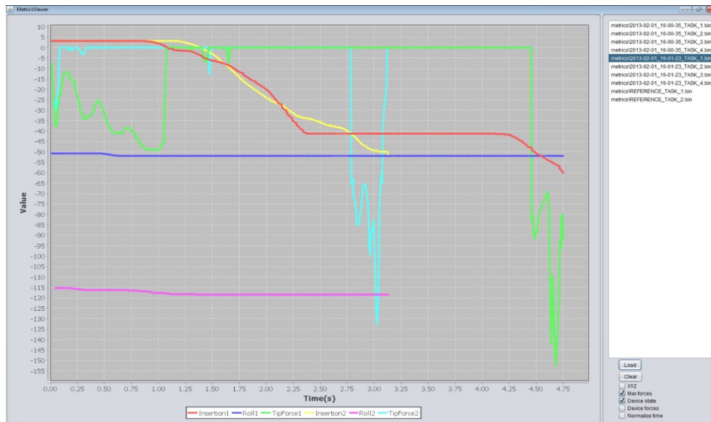
Figure 4.16: The metrics analysing tool. Visually compares two completions of the same task in terms of device insertion in cm (red and yellow), roll in angles (blue and magenta) and the force exerted on the tip (no units, green and cyan).
