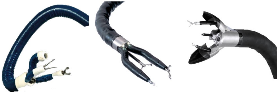
Figure 4.2: Prototypes of NOTES endoscopes. On the left, Cobra by USGI medical. In the middle, a concept device by Olympus Medical Systems. On the right, Anubis by Karl Storz.
