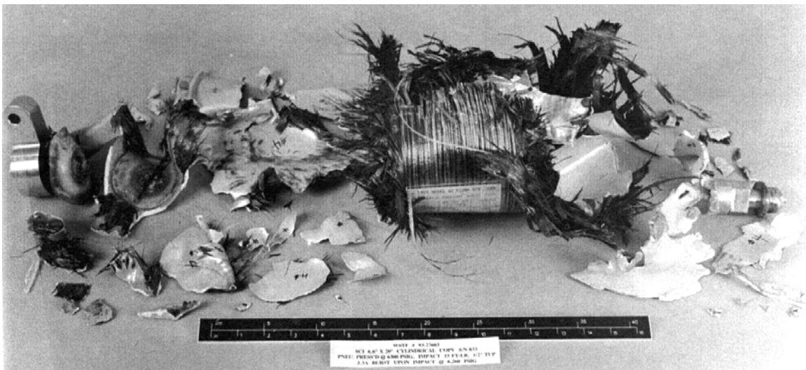
Figure 9. Pneumatic burst of a COPV.
