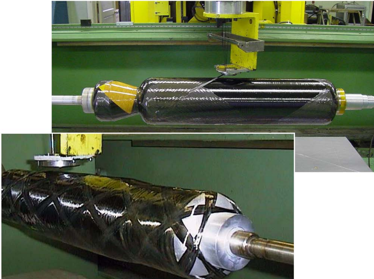
Figure 5. Fabrication of filament wound pressure vessels with hoop and helical layers.
