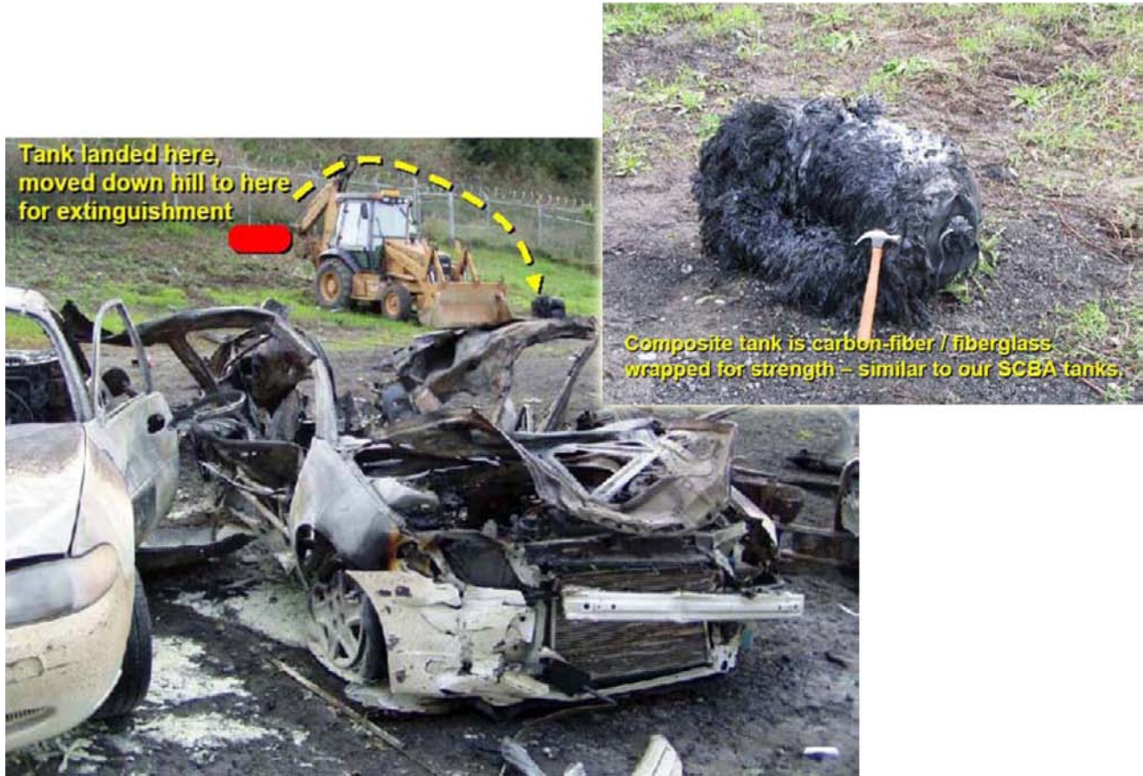
Figure 10. Automotive application failure in Malaysia.
