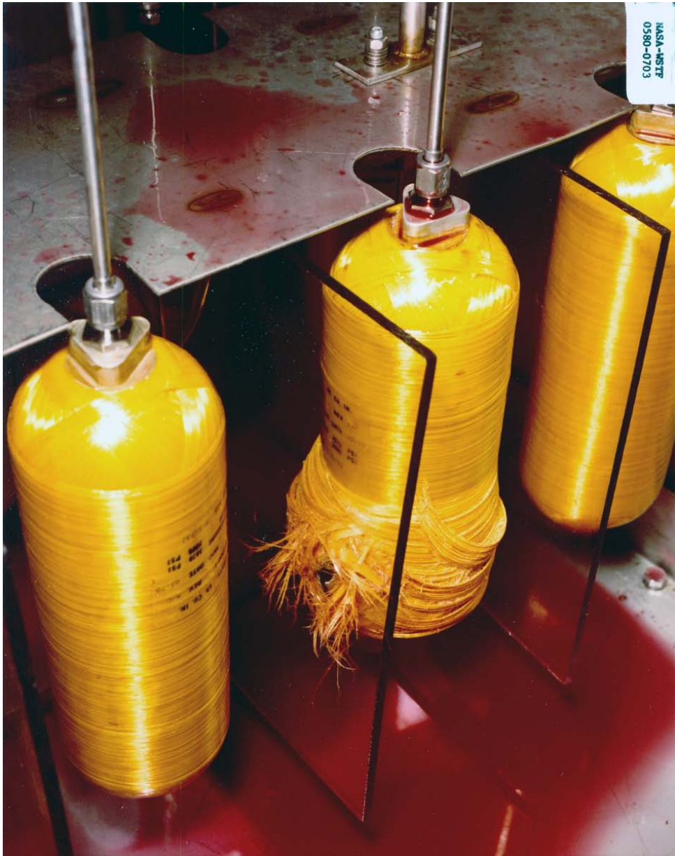
Figure 7. Stress rupture testing and a hydraulic failure.
