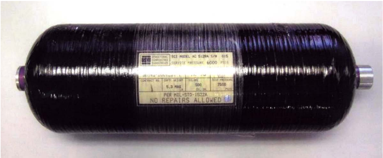
Figure 3. Carbon fiber COPV, 6×18 in.
