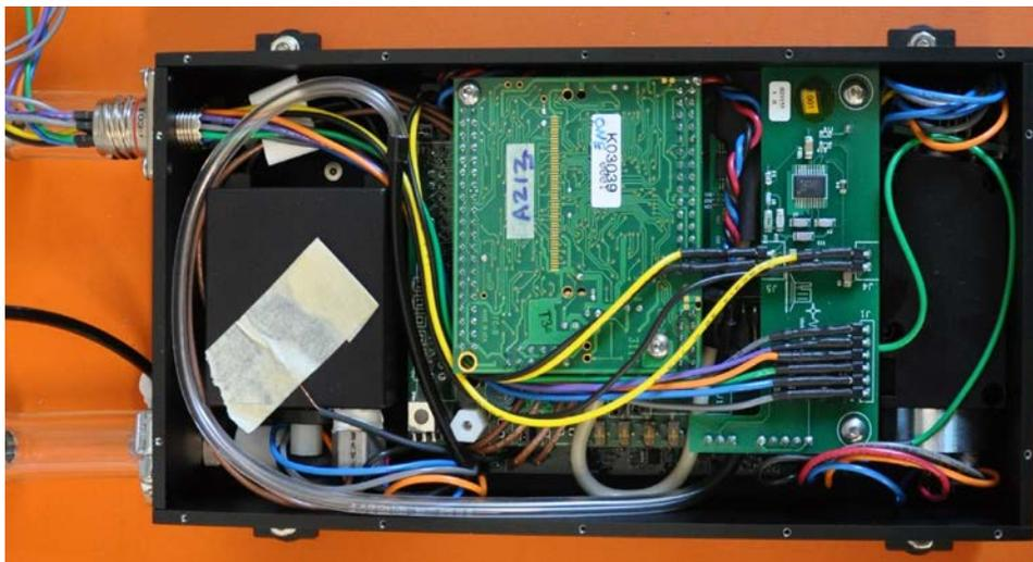
**Figure 7. Integrated Version 2.0 sensor.** *Optical and electronic layout after full conversion to 2.0 architecture. An RS-485 bi-directional interface and power supply board compatible with the APLSS 2.0 system has been added.*
