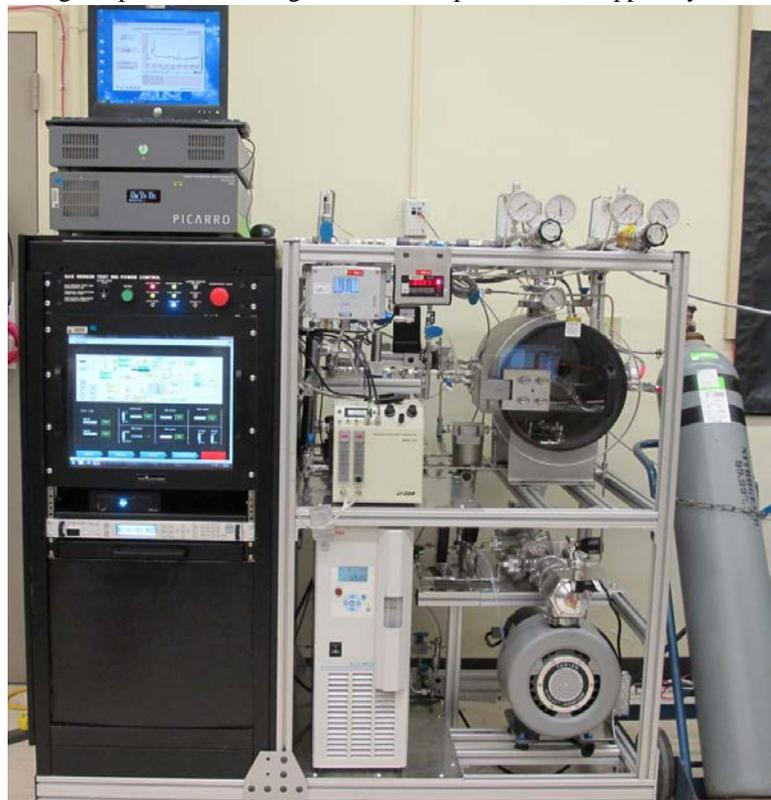
**Figure 15. NASA JSC Gas Sensor Test Stand.**
