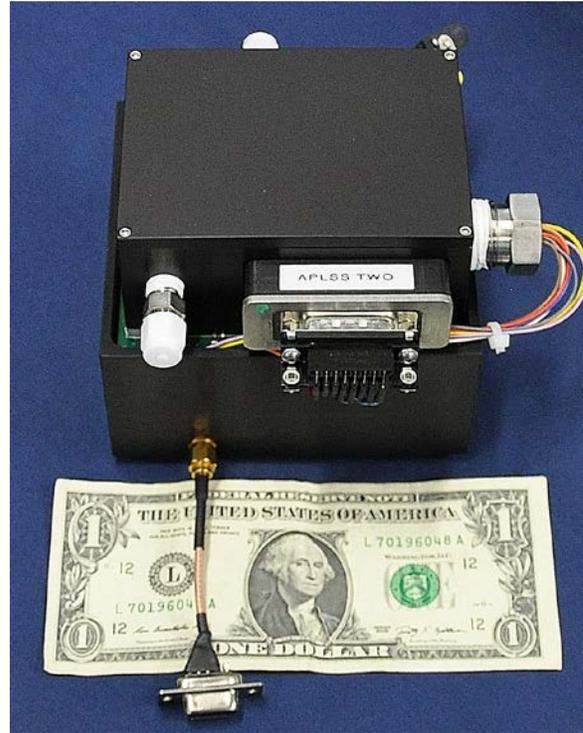
**Figure 1. Version 1.0 APLSS Optical Sensor.** The nearly cubic shape met the footprint requirements sought at the time of the development.
