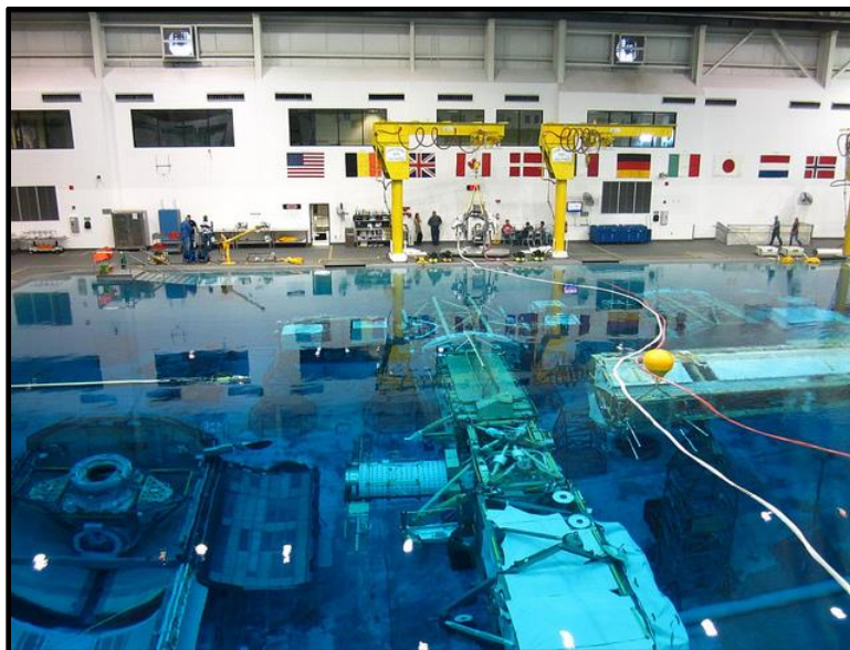
Figure 4. The Neutral Buoyancy Laboratory (NBL) with the Space Shuttle cargo bay (left) and ISS modules (right) in August, 2011 (photo courtesy of NASA).
