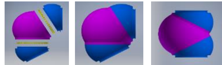
University of Maryland: 3D Printing of Spacesuit components (pictured: 3-element wedge for elbow)
