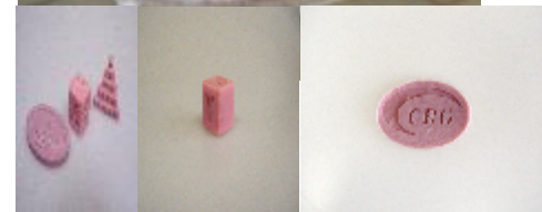
FDM prints using reclaimed anti-static bagging film with reversible cross-linking additive (image from Cornerstone Research Group) 16
