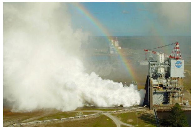
Fig. 8. RS-25 hotfire test at Stennis Space Center.
