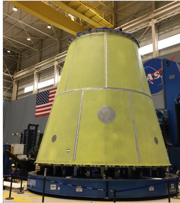
Figure 6 EM-1 LVSA undergoing final priming prior to foam application.
