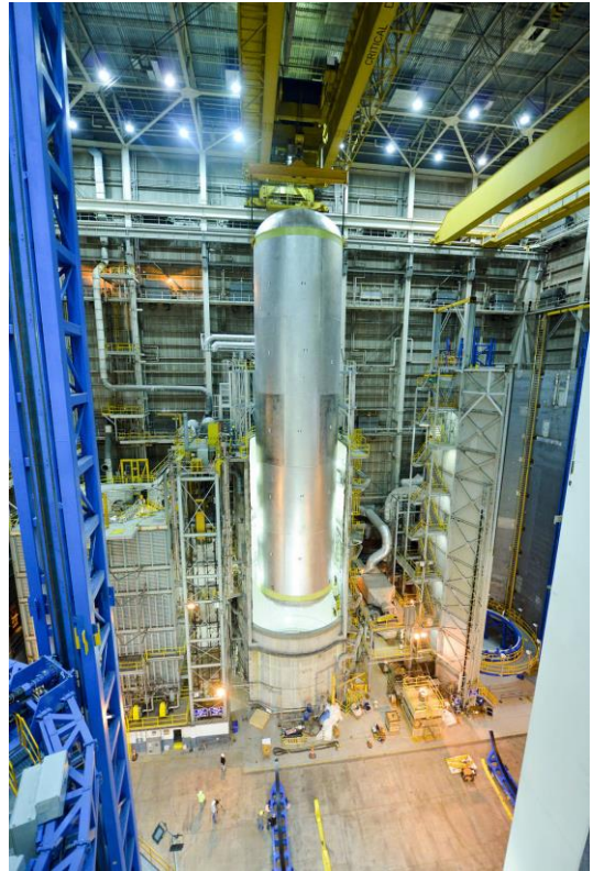
Figure 2 Test article of liquid hydrogen tank of the SLS core stage
