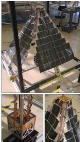
Figure 2. Single-side, deployed LISA-T omnidirectional configuration prototype. The complete, deployed power system and antenna were stowed in 0.6U.
