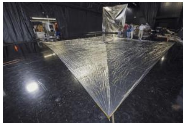
Figure 1. 86 square meter test sail deployed horizontally during a test at NASA MSFC. A half-scale sail hangs vertically in the background.
