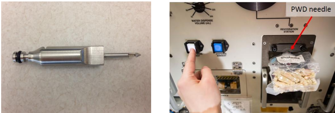
Figure 1. Left image: the PWD needle. Right image: the PWD needle being used to rehydrate a food package.
