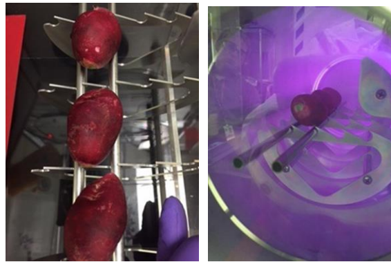
Figure 2. Radishes exposed to plasma at 0.80 mbar pressure.
