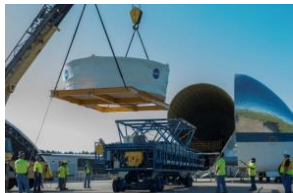
Figure 10 Loading of the OSA test article for delivery to Colorado
