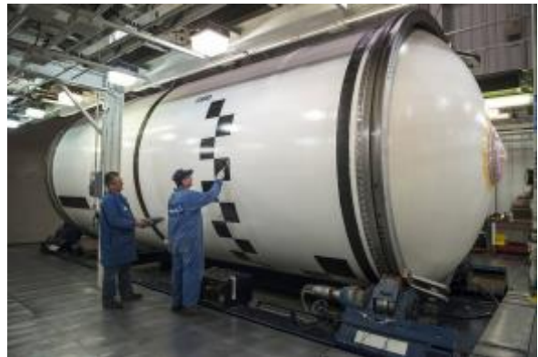
Figure 4 Technicians applying photogrammetric markings on completed segments for the five-segment solid rocket booster motors for the first integrated mission of SLS.
