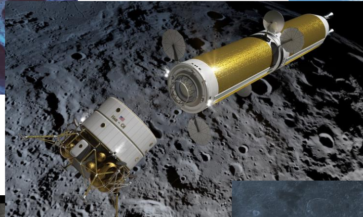
Reusable Lunar Transfer Vehicle uses Single 75 klb f NTR Engine – SEI (1990 - 91)
