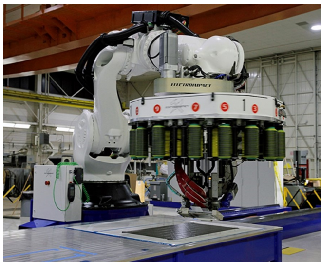
Fig. 1. NASA Langley Research Center’s carbon fiber fabrication robot ISAAC (Integrated Structural Assembly of Advanced Composites).
