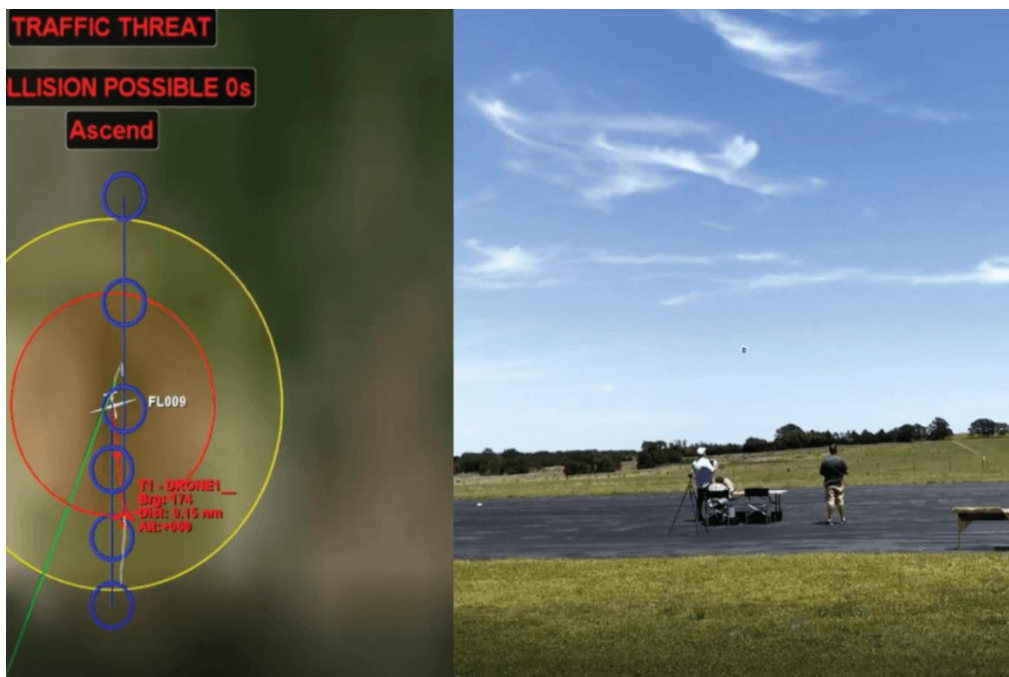
Fig. 20. ADS-B DAA Flight 5 on May 2017; commands maneuver to safely avoid the collision.
