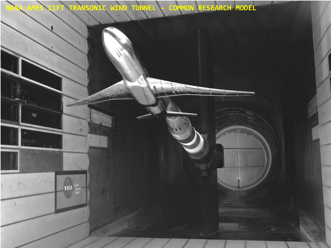
Fig. 1 Test of NASA's Common Research Model in the NASA Ames 11-ft Transonic Wind Tunnel.
