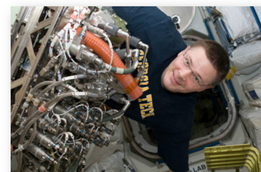
Astronaut installing Sabatier system
