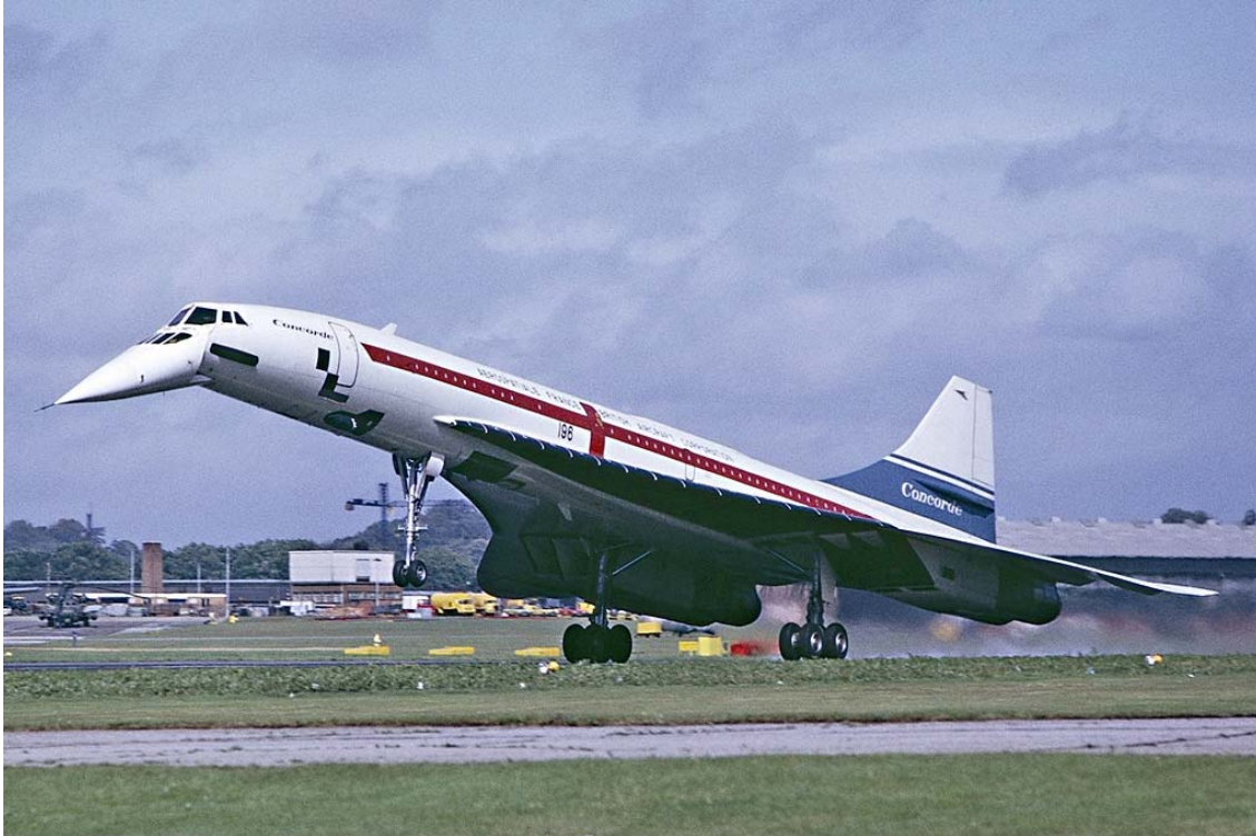
Figure 6: Concorde Droop Nose [23]
