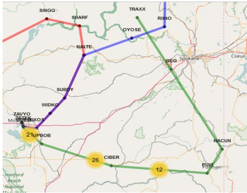
Figure 6. Map of speed increases during arrival scenarios for UPBOB1 route with Cross-FAF time-based operations
