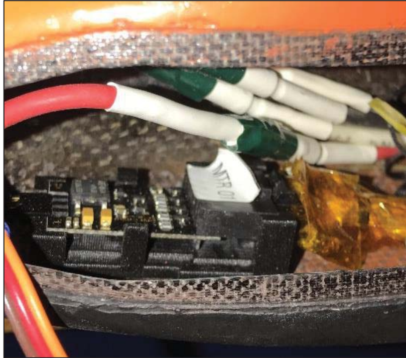
Figure 10. Motor 1 Nacelle w/Integrated Serial Link
