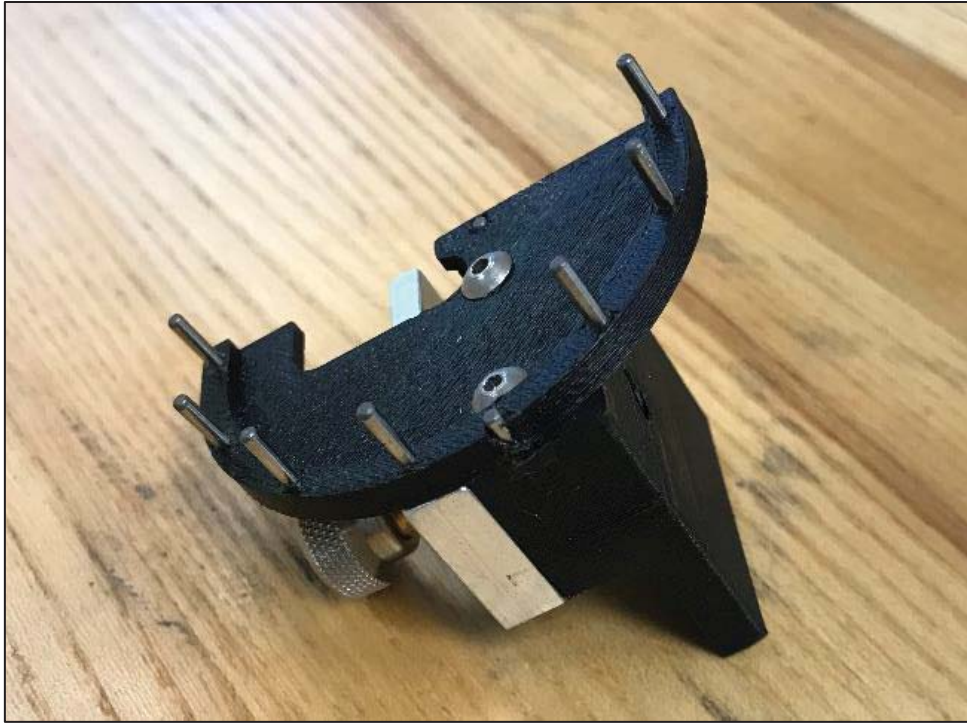
Figure 14. Alpha/Beta Potentiometer Calibration Tool (-30°, 0°, 30°)
