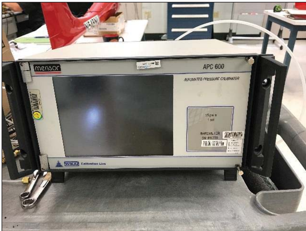
Figure 15. Pitot Probe Calibration Tool (Static/Dynamic)
