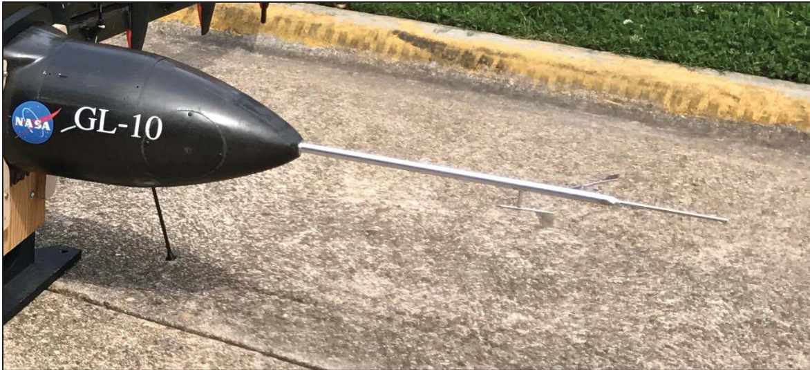
Figure 12. SpaceAge Controls Alpha/Beta Pitot Tube
