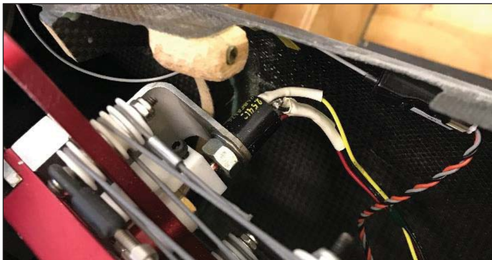
Figure 13. Tail Actuator Arm w/Integrated Potentiometer
