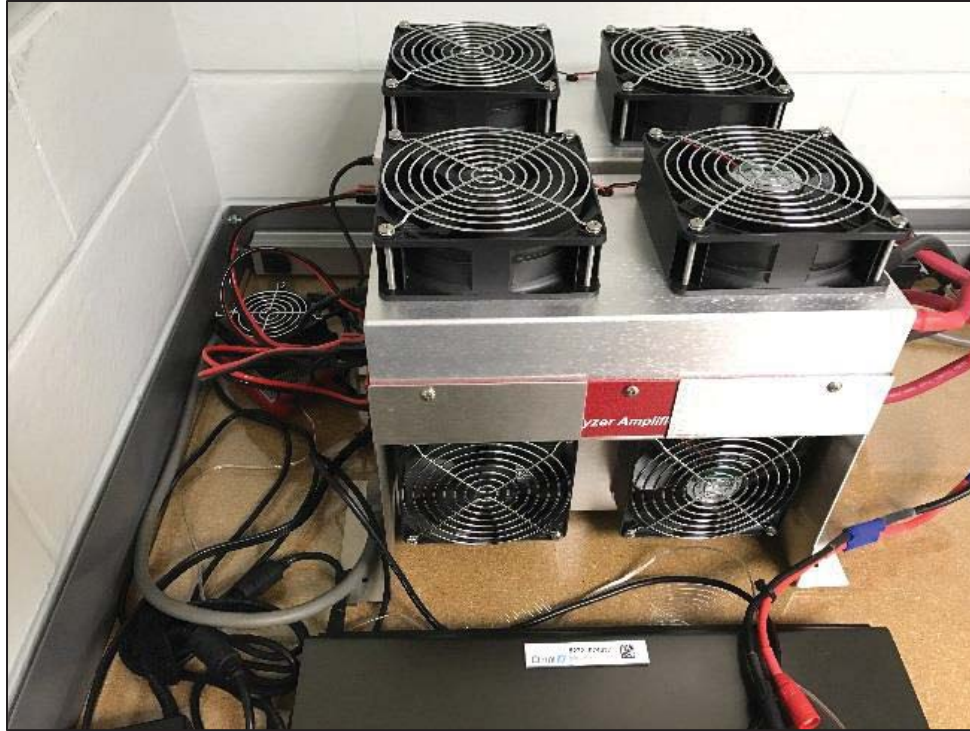
Figure 16. 150A Current Sensor Calibration Tool
