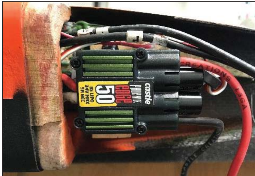
Figure 9. Motor 1 Nacelle w/Integrated ESC
