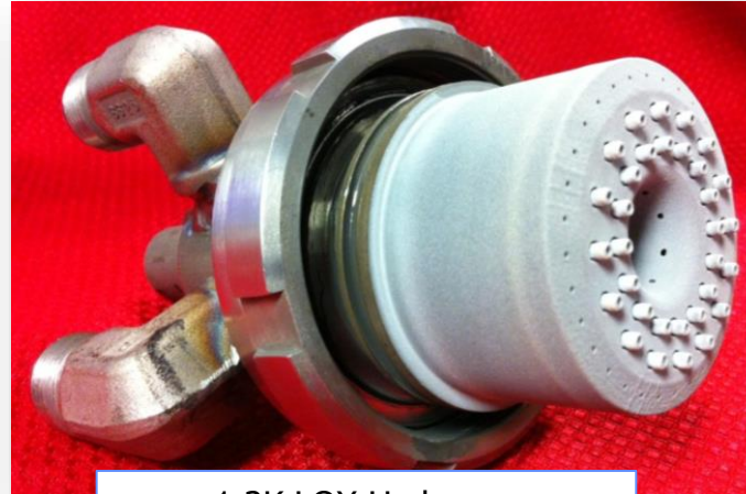
1.2K LOX Hydrogen First Tested June 2013 >3900 sec hotfire
