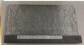
Arc-Deposition of MCC Liner, Inco 625
