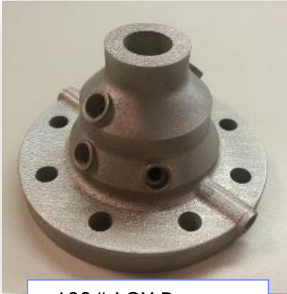
100# LOX Propane Injector Built 2012 Tested Nov 2013
