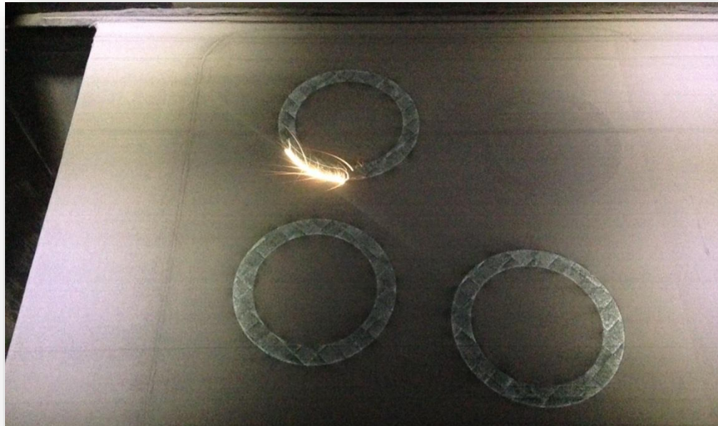
SLM GRCop-84 Copper-alloy Material in the As-built Condition (ASTS, Huntsville)
