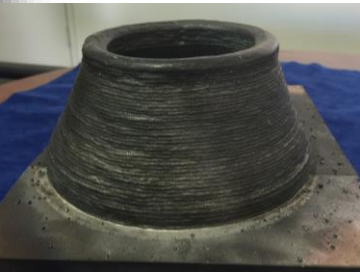
Large Scale Deposition: Blown Powder and Arc Deposition
