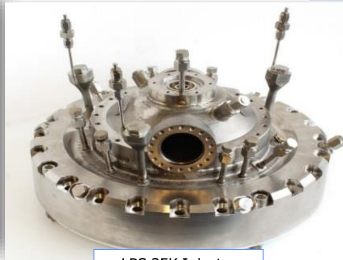
LPS 35K Injector Welded Manifolds Tested Nov 2015
