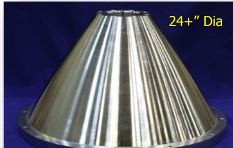
Large Scale Deposition: Blown Powder and Arc Deposition
