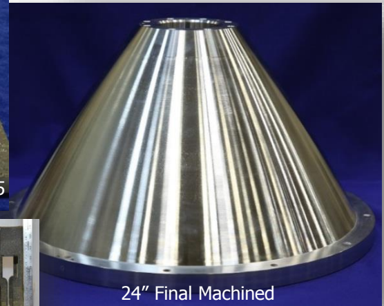
Arc-Deposition of MCC Liner, Inco 625
