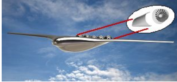
Figure 1. Hybrid wing body vehicle with boundary layer ingesting propulsion from a system study 3 .
