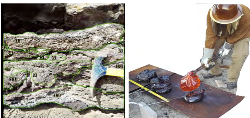
FIGURE 3. Mapping and measurement of welded lava spatter at COTM compared to simulated spatter experiments conducted at the Syracuse Lava Project.
