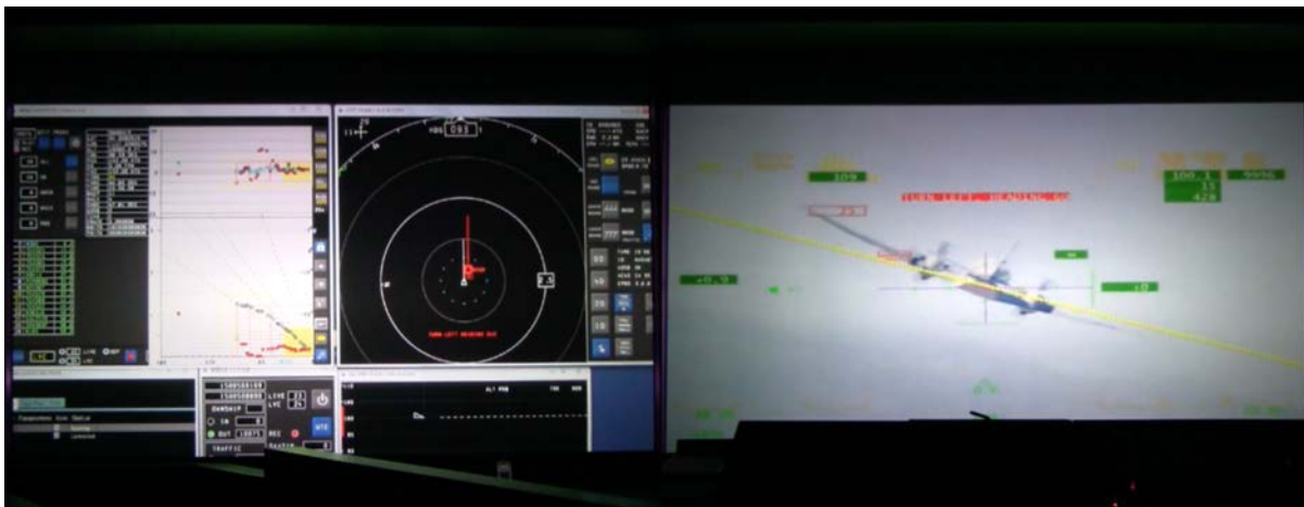
Figure 9. Streaming Video. The side-by-side streaming video of the Ikhana ball camera and the DAA traffic display as shown in FFC during the live ACAS flight.
