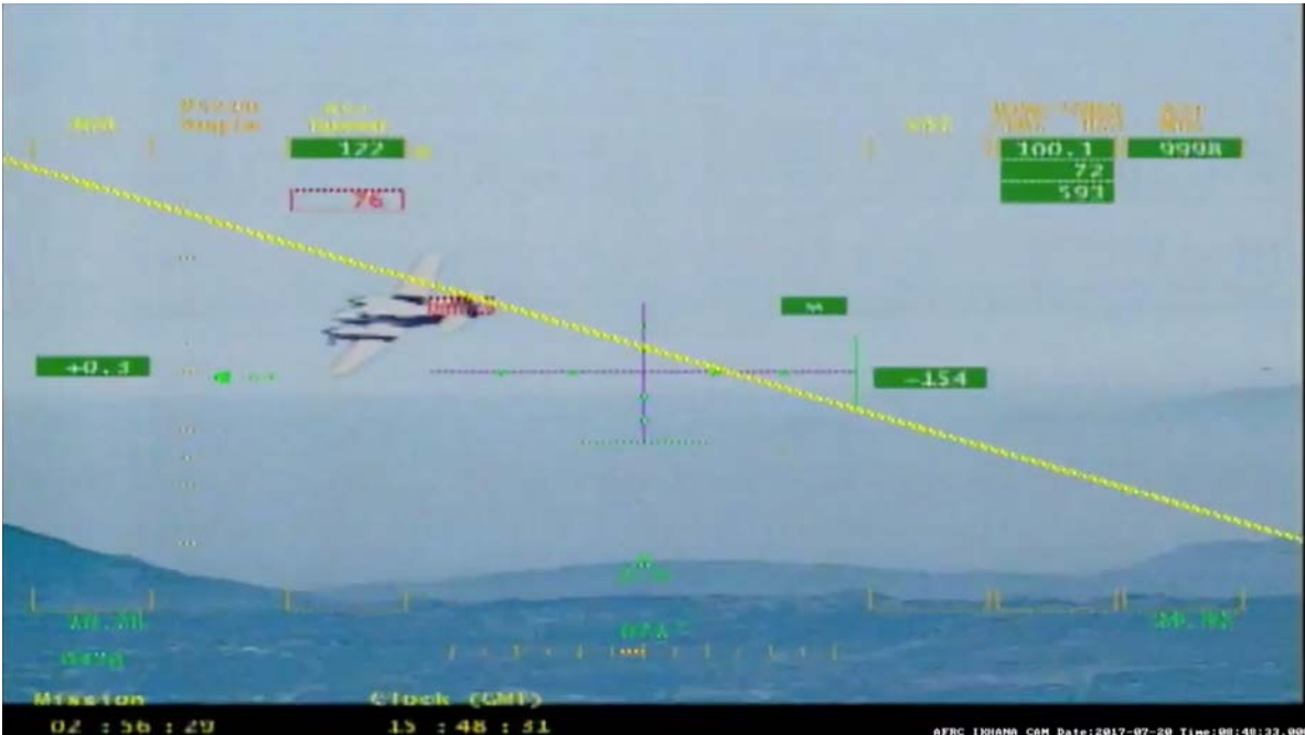
Figure 4. Ikhana Video Feed. Video from the Ikhana nose camera with embedded flight information.
