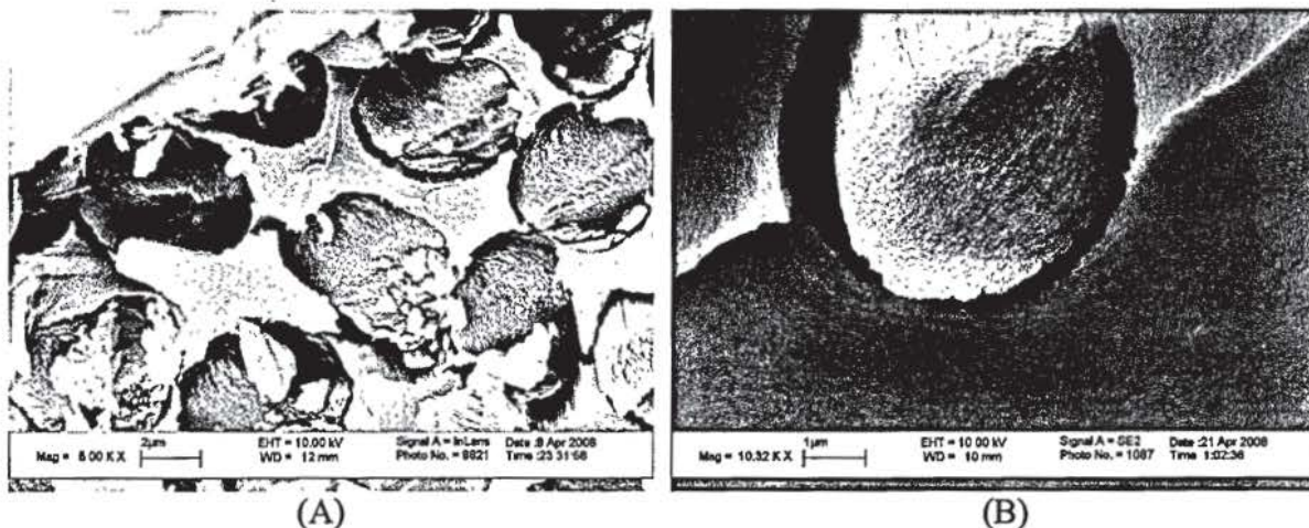
Figure 17. SEM pictures of the PMC showing no MWCNTs in the sample taken from the (A) middle and (B) outlet side of the RTM Tool (GSFC-01-6).
