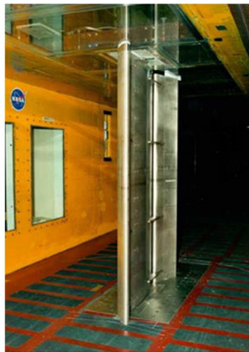
Figure B.8.—McDonnell Douglas Aerospace multi-element airfoil (MEA). (a) Two-dimensional cross-section geometry. (b) Test model installed in the Icing Research Tunnel (IRT).
