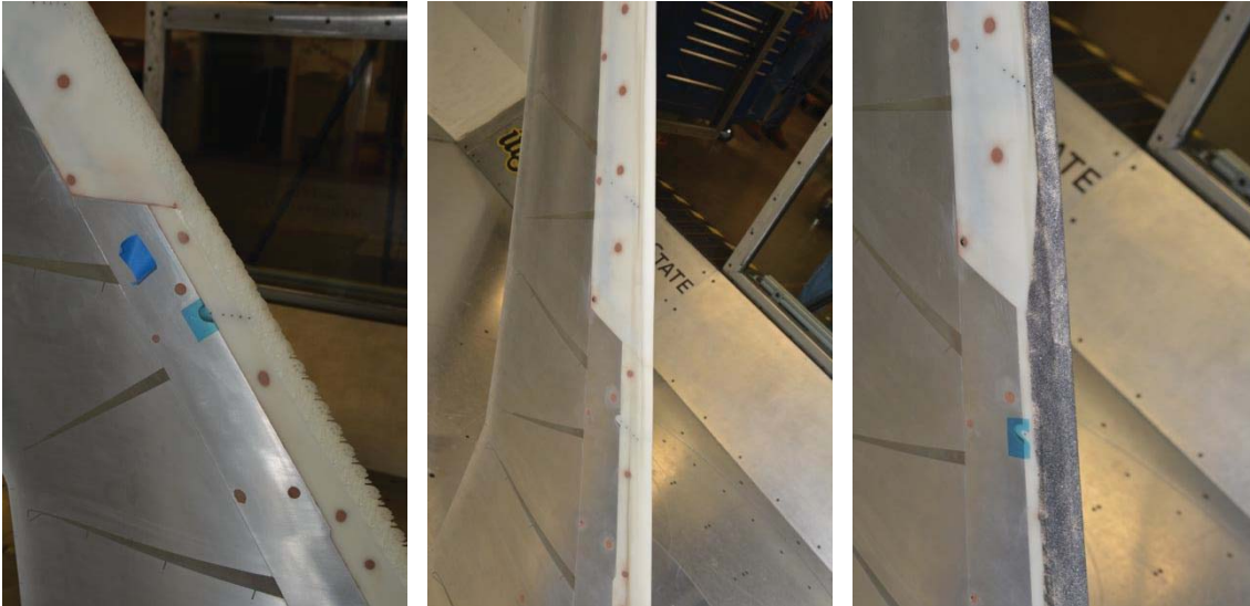
Figure 3: Shown left to right - High fidelity, 2D smooth, and 2D smooth + grit artificial ice shapes installed on the 8.9% scale CRM wing.
