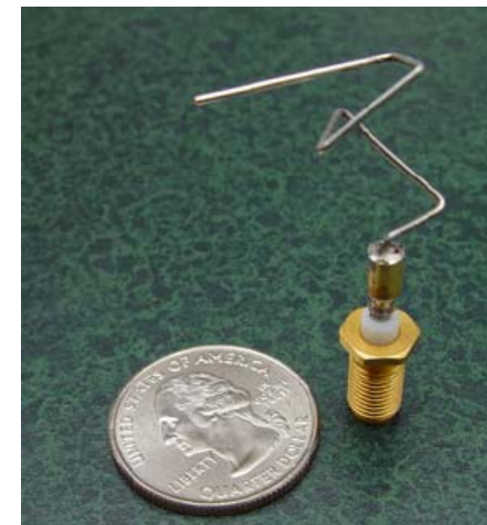
NASA ST5 spacecraft antenna evolved to optimize the radiation pattern
