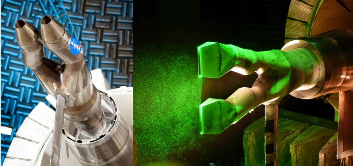
Figure 3 Pictures of acoustic testing of twin, single-stream, round nozzles (left), and of PIV testing of twin rectangular nozzles (right).
