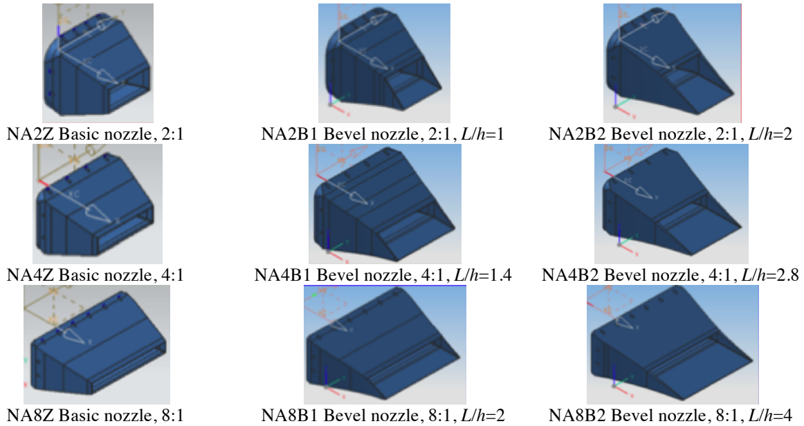
Figure 2 Gallery of Extensible Rectangular Nozzles.
