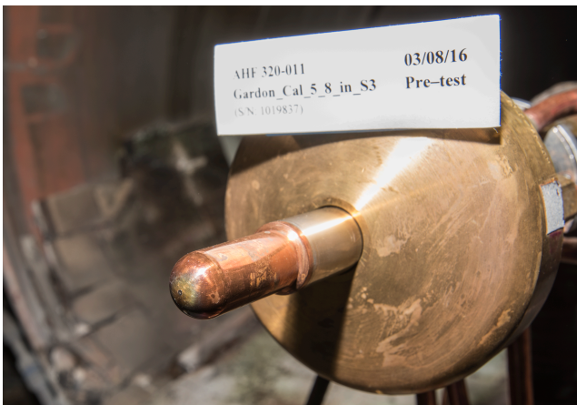
(c) 15.9-mm hemisphere probe, Gardon gage
