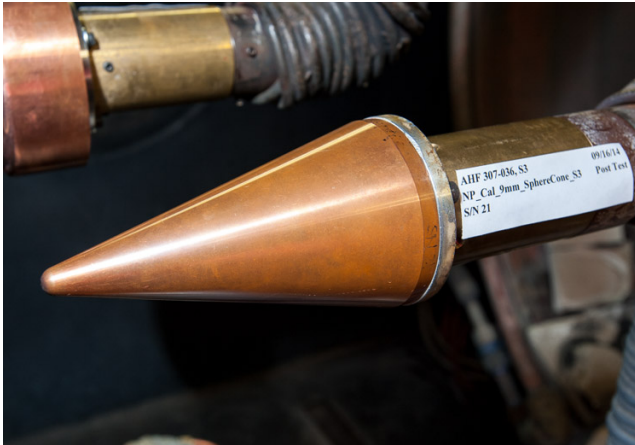
(a) 9.1-mm sphere-cone probe, null-point gage
