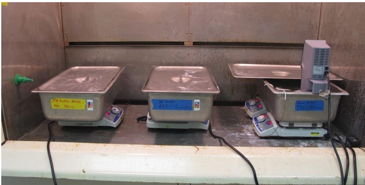
Figure 9. Test panels soaking in citric acid.
