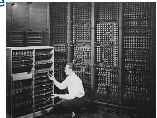
Replacing a bad tube meant checking among ENIAC's 19,000 possibilities.
