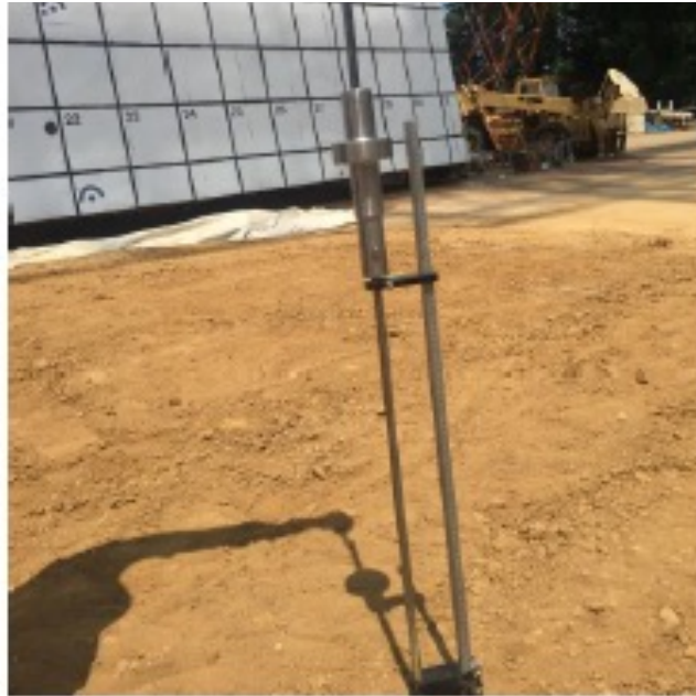
Figure 10. Photograph and schematic of the Dynamic Cone Penetrometer.
