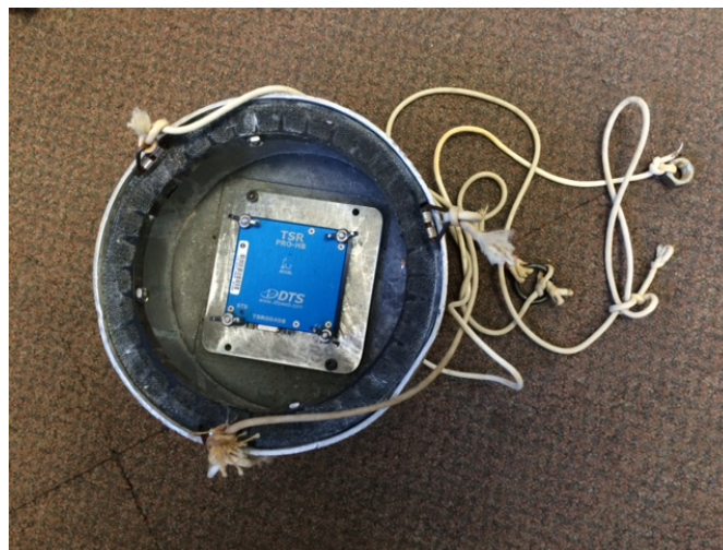
Figure 9. Ball penetrometer with TSR shock recorder.
