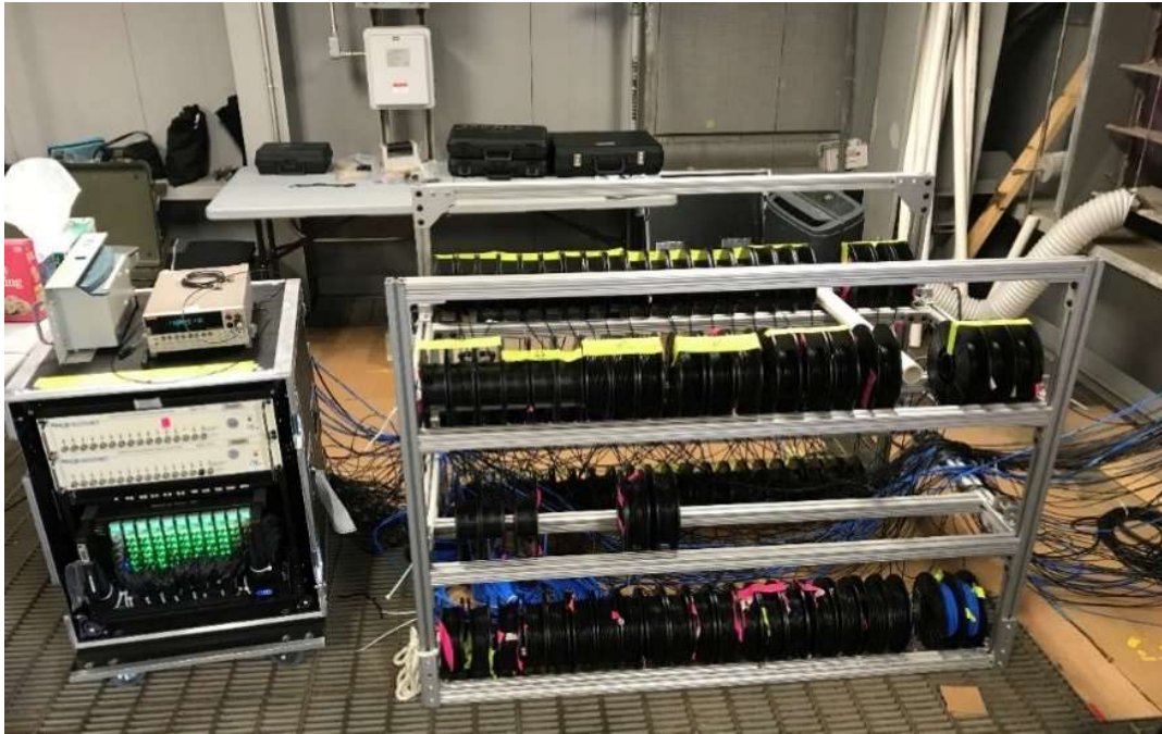
Figure 6: Accelerometer Cable Spools, DC Signal Conditioners, and Data Acquisition Chassis
