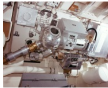
Skylab Materials Processing Facility Multipurpose Furnace System
