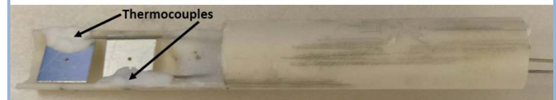
Cut piece of alumina tubing showing sample and thermocouple placement. (Less cement, different design, larger samples, can obviously be implemented.)
