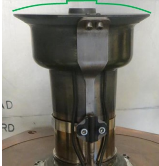
Figure 10.—Exaggerated illustration of crowning of ASC-E3 #1 and #2 across the heat collector face.
