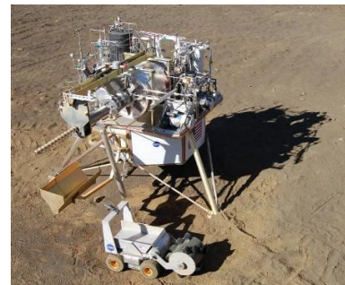
PILOT H 2 Reduction Water Electrolysis Bucketdrum Excavator
