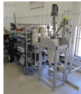
Soil Processing Module 10kg per batch; 5 kg/hr 0.15 kg/hr H 2 O (3% water by mass)
