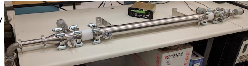
Initial set-up of electrostatic precipitator in a flow-through test
