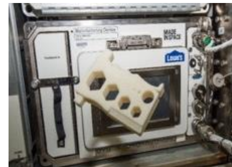
Additive Manufacturing Facility (AMF) on ISS developed via SBIRs with Made in Space, Inc.
