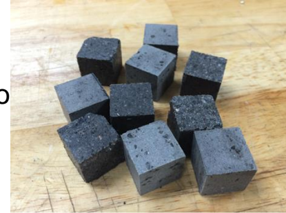
Standard 2-inch cube compression test specimens
