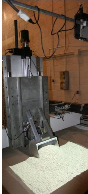
Excavation force determination with soil surface 3D measurement using structured light stereography
