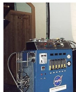
CO 2 Electrolysis (GRC) [Tested under conference conditions]
