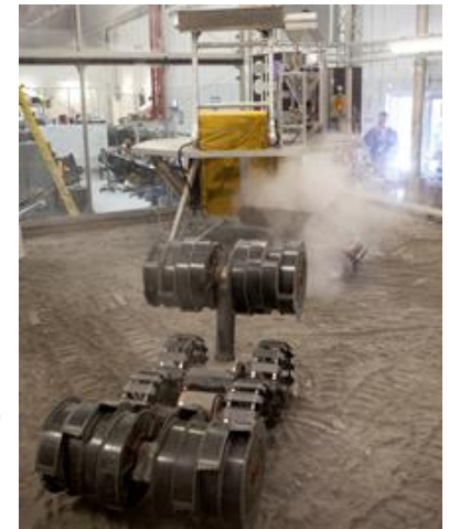
RASSOR (Regolith Advanced Surface Systems Operations Robot) excavator delivering loose soils
