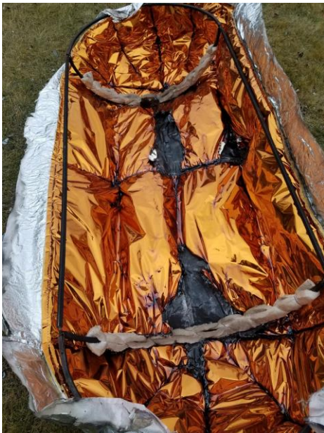
FIGURE 23: TYPICAL DOUBLE SHELTER INTERIOR POST-TEST CONDITION.
