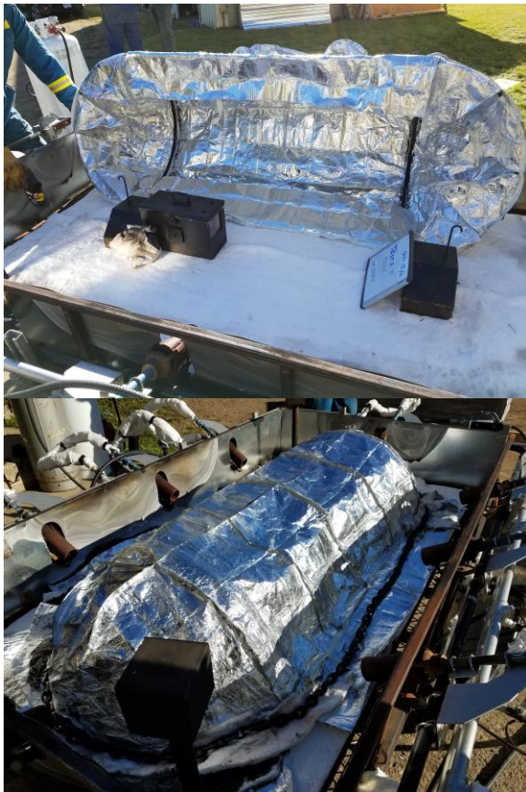
FIGURE 5: FULL SCALE SHELTER TEST APPARATUS WITHOUT ENCLOSURE. INSTRUMENTATION (TOP), AND DEPLOYED TEST ARTICLE (BOTTOM).
