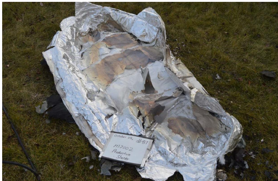
FIGURE 19: TYPICAL M2002 INTERIOR POST-TEST CONDITION.
