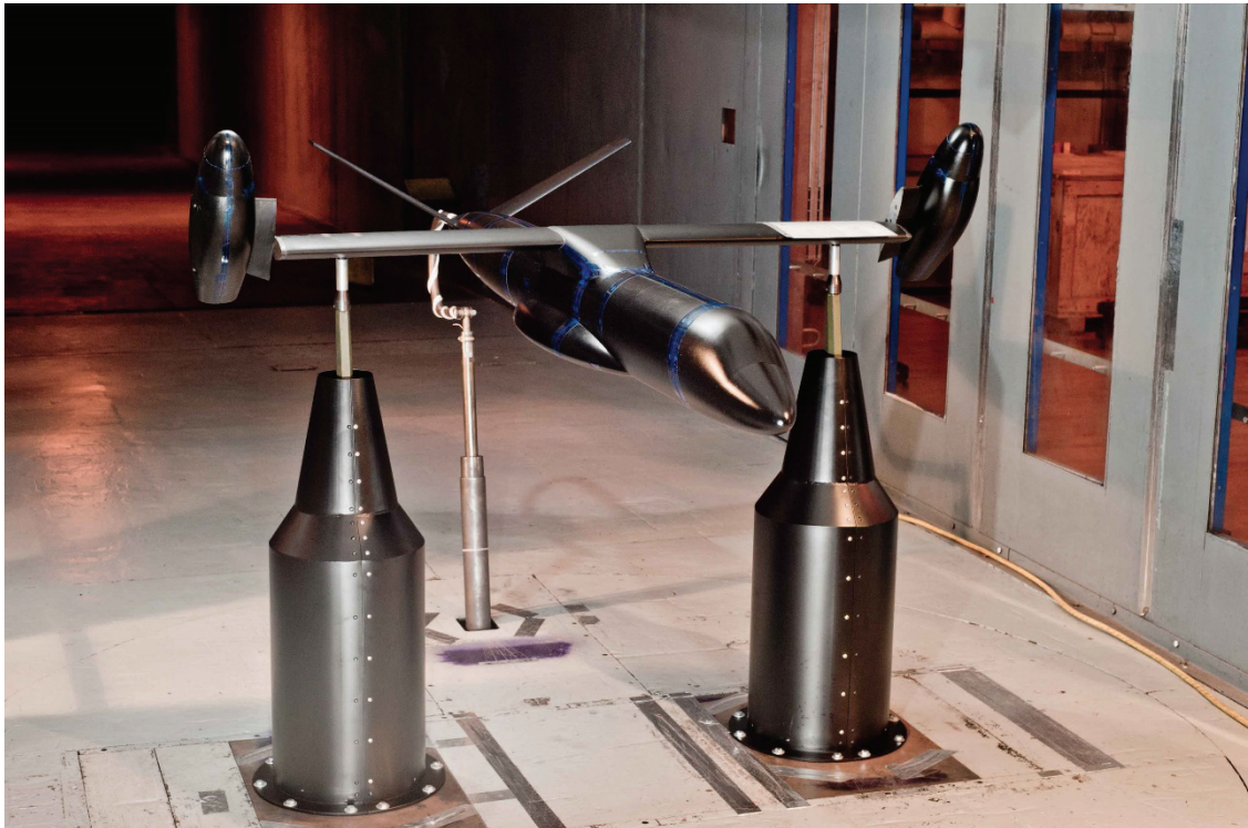
Figure 13: The L60 model configuration mounted inside the wind tunnel with round fairings.
