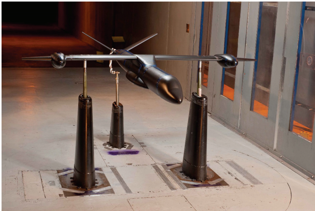
Figure 5: The L00E model configuration mounted inside the wind tunnel with aerodynamic fairings.
