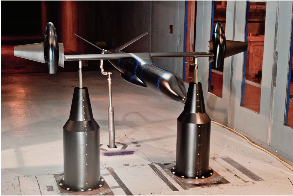
Figure 12: The L95E model configuration mounted inside the wind tunnel with round fairings.
