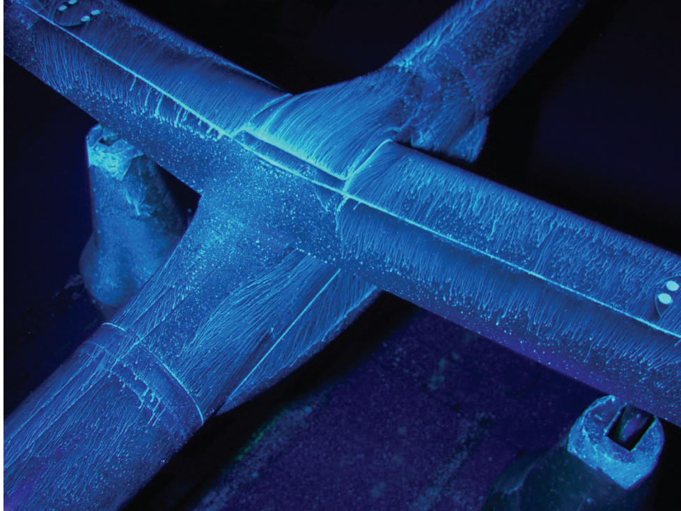
Figure B-119: LS12 flow visualization over wing.
