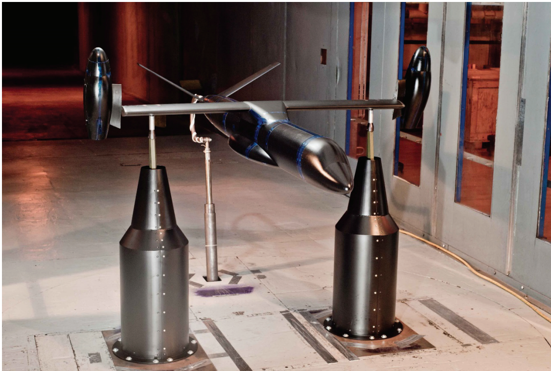
Figure 14: The L75 model configuration mounted inside the wind tunnel with round fairings.
