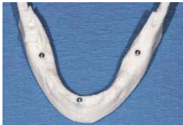
Figure 1: Model 1: Radiopaque acrylic resin model of edentulous mandible with three mini-implants in place.
