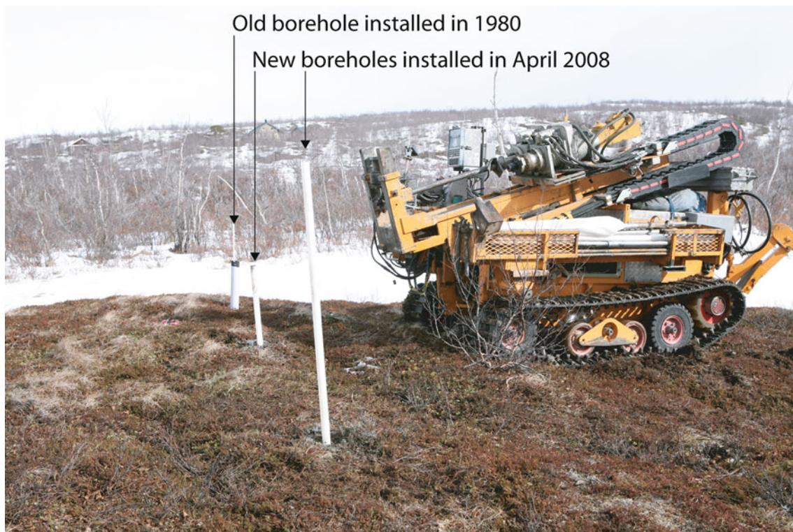
Fig. 2 The old and new boreholes at the Kursflaket mire 3 km east of Abisko (Photo: J. Åkerman)
