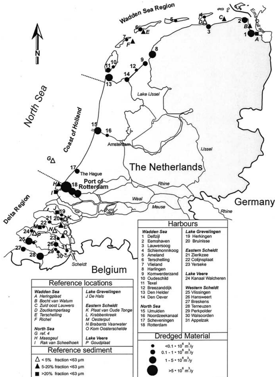
Fig. 1. Harbors and reference locations along the Dutch coast where sediments were sampled during the 1999–2000 survey. Also indicated are the annual volume of dredged material and the sediment texture at the reference sites
