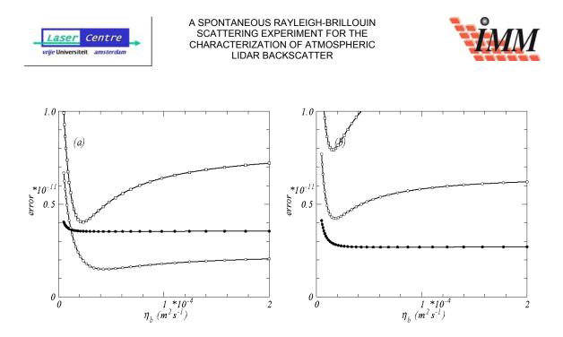
Figure 9-14: Dry air, spontaneous Rayleigh-Brillouin scattering. (a) Error of the S6 model as a function of  $\eta_b$ , dots, open circles and open squares, p = 1, 2, 3 bar, respectively.
