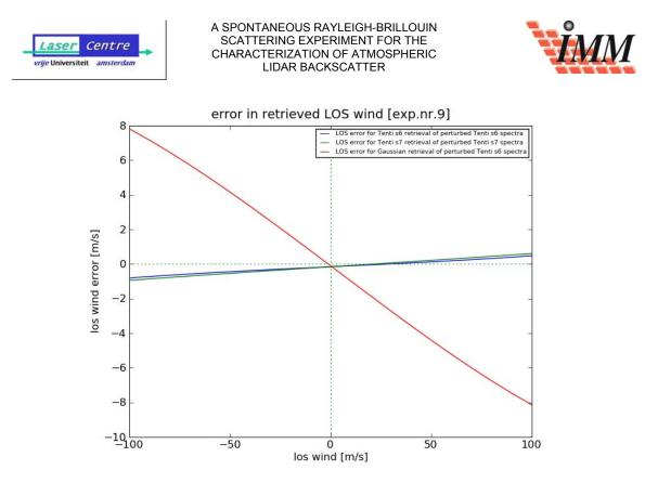
Figure 11-29: LOS wind error calculated from the residuals from experiment 9 (pressure 1008 hPa).
