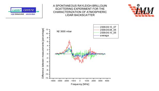
Figure 7-13: Residual plots of the difference between the measurements (and the average), in percentage of the amount of (normalized) signal.
