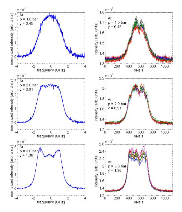
Figure 8-4: Experimental results on Coherent Rayleigh Brillouin scattering at 532 nm for various pressures in Ar. On the right raw data, on the left averaged data.
