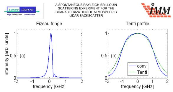
Figure 3-14: (a) Calculated transmission function of the Fizeau wedge (Eq.(3.5)) with properties from Table 3.1. (b) Calculated Tenti profile and the convolution with the calculated transmission function as (a).
