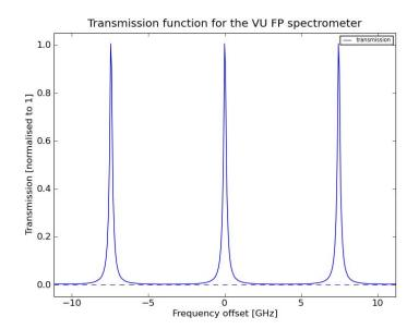
Figure 11-3: Airy function used to model the transmission of the VU FP spectrometer. ESA-TENDER AO/1-5467/07/NL/HE
