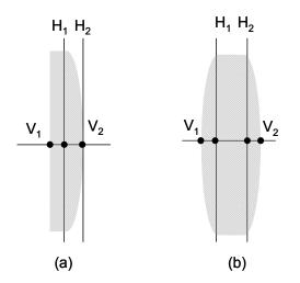
Figure 3-5: Primary  $H_1$  and secondary  $H_2$  principal planes of a plano-convex (a) and a biconvex lens (b). The thickness of the lens dI or  $V_1V_2$  is not negligible, because the actual focal distance f of the lens is measured relative to the principal planes.
