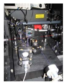
Figure 5-5: Picture of the enhancement cavity. In blue is depicted the path of the main laser beam, in red is depicted the path of the reference laser. The light of the reference laser goes from right to left.
