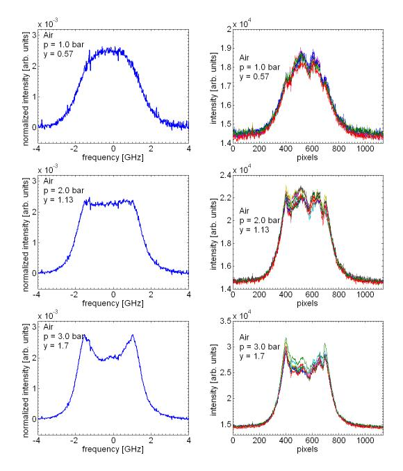
Figure 8-5: Experimental results on Coherent Rayleigh Brillouin scattering at 532 nm for various pressures in Air. On the right raw data, on the left averaged data.
