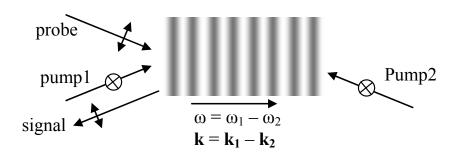
Figure 3-1: Coherent Rayleigh-Brillouin scattering. Light is Braggdiffracted on the gas density fluctuations created by a laser-induced electrostrictive grating. The optical dipole force pushes the molecules towards the high field intensities of the optical grating.
