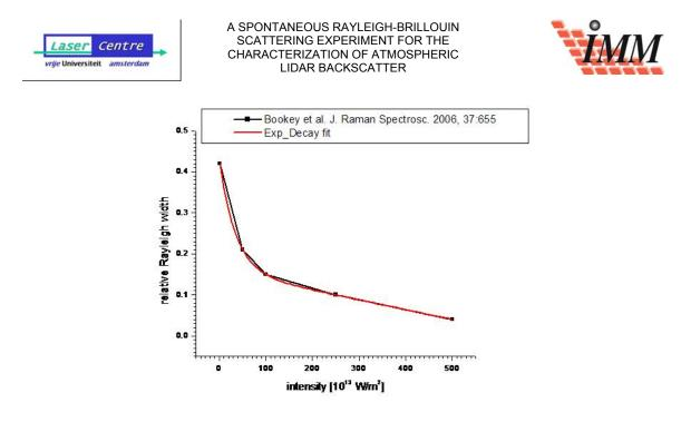
Figure 3-18: Relative Rayleigh scattering linewidth as a function of the pump intensity. Significant spectral narrowing of the CRS spectrum occurs for increasing pump intensity larger than  $10^{14}$  W/m<sup>2</sup>.
