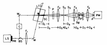
Figure 4-2: Setup used by Lao et al [48] to record RBS. The scattered light is filtered using 3 pinholes ( $S_1$ ,  $S_2$  and  $S_3$ ) and a set of 2 lenses ( $F_2$  and  $F_3$ ). The choice of scattering angle is 60°.
