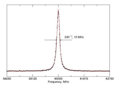
Figure 5-13: Measured instrument function, for the Fabry-Perot detector, PMT and electronics. Black dots: the experimental results (for the laser). Red line: Fit of the results.
