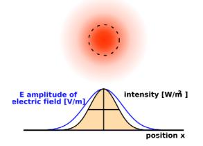
Figure 5-18: Geometrical shape of a Gaussian beam. This is the shape of the light intensity accepted by the Fabry-Perot etalon. Figure is taken from [51].
