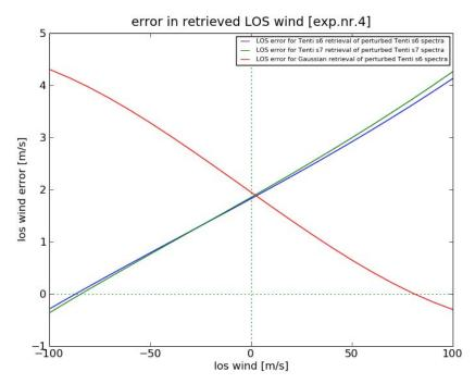
Figure 11-24: LOS wind error calculated from the residuals from experiment 4 (pressure 500 hPa). Note that this experiment clearly suffered from some Mie contamination.
