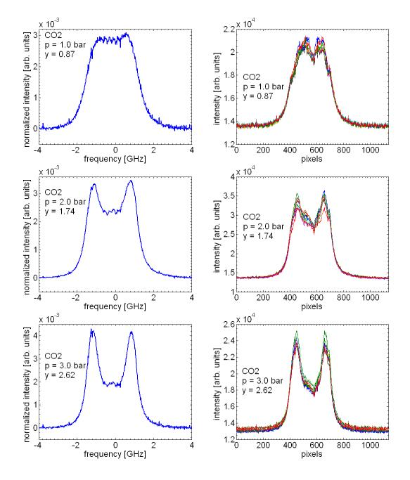
Figure 8-3: Experimental results on Coherent Rayleigh Brillouin scattering at 532 nm for various pressures in  $CO_2$ . On the right raw data, on the left averaged data.
