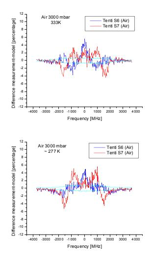
Figure 7-41: Residual plots of the difference between the measurement and the model, in percentage of the amount of (normalized) signal. The uncertainty on the intensity is shown by the two curves in light blue.
