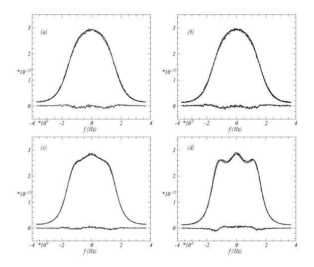
Figure 9-13: Dry and humid air, spontaneous Rayleigh-Brillouin scattering. (a) dry air p = 1 bar,  $\eta_b = 1.0881 \times 10^{-5}$  kg m<sup>-1</sup>s<sup>-1</sup> (the literature value); (b) air with 100% humidity, p = 1 bar,  $\eta_b = 1.088 \times 10^{-5}$  kg m<sup>-1</sup>s<sup>-1</sup>; (c) dry air, p = 2 bar,  $\eta_b = 2 \times 10^{-5}$  kg m<sup>-1</sup>s<sup>-1</sup>. (d) dry air, p = 3 bar,  $\eta_b = 2 \times 10^{-5}$  kg m<sup>-1</sup>s<sup>-1</sup>.
