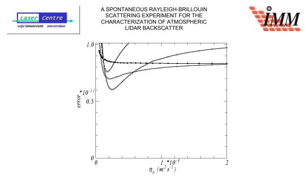
Figure 9-8: N<sub>2</sub> coherent Rayleigh-Brillouin scattering. Same as Figure 9-7(d), but now the error is for the Tenti S7 model. There are two different experiments for p = 3 bar. For pressures  $\ge 2$  bar, the S7 model has significantly larger errors.
