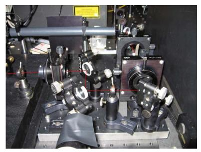
Figure 5-22: Light cleaning stage for the laser beam. The path of the beam is marked in red.
