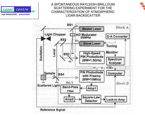
Figure 4-1: Experimental layout of the Superheterodyne detection system by Tanaka and Sonehara [45] for measuring RB-scattering at extremely high resolution.
