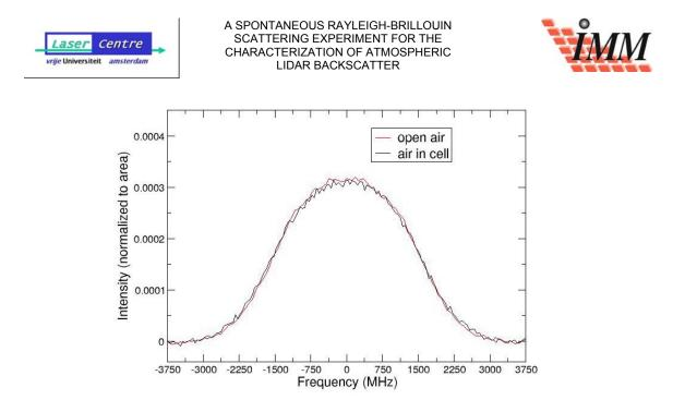
Figure 6-5: Normalized (to the area) spectra of the SRBS in air. Red curve: the scattering from open air, without the scattering cell. Black curve: the scattering from air from inside the scattering cell, at atmospheric conditions. Both curves coincide. The signal to noise of both measurements is comparable, and they took roughly the same amount of time to measure (3 hours).
