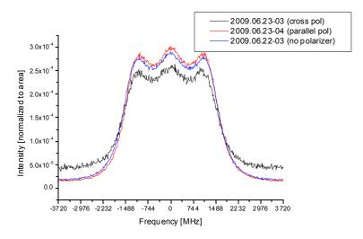
Figure 7-45: Spectra of  $O_2$  gas at 3500 mbar and ambient temperature (the y value is 1.8154). The black curve is with a polarizer at a 90° angle with respect to the laser polarization, the red curve is with the polarizer at a 0° angle with respect to the polarization of the laser, and the blue curve is a measurement without polarizer.
