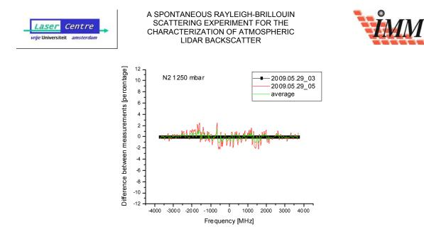
Figure 7-8: Residual plots of the difference between the measurements (and the average), in percentage of the amount of (normalized) signal.
