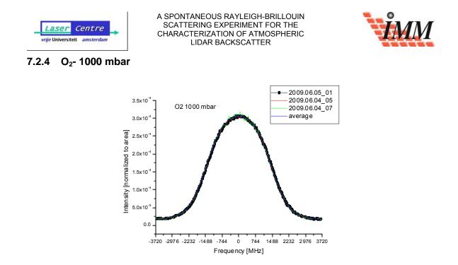
Figure 7-20: To compare different measurements, in which the intensity may vary, the intensity scale is normalized to area equal to one.
