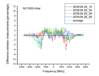
Figure 7-15: Residual plots of the difference between the measurements (and the average), in percentage of the amount of (normalized) signal.
