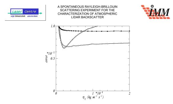
Figure 9-16: Dry Air, coherent Rayleigh-Brillouin scattering. Same as Figure 9-15 but now for the S7 model.
