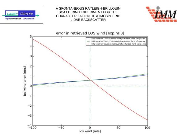
Figure 11-23: LOS wind error calculated from the residuals from experiment 3 (pressure 504 hPa).
