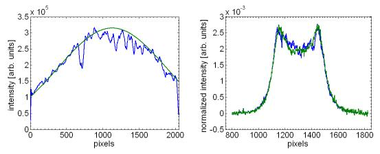
Figure 3-15: (a) Amplitude variation of each pixel in the photodiode array of the Fizeau spectrometer using the broad-band pump laser at 532 nm (blue line) and Gaussian fit to the envelope of the amplitude variation (green line). (b) Measured CRBS spectra with (green line) and without correction (blue line). Each measurement is averaged over 500 shots.
