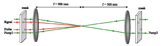
Figure 3-3: The three-dimensional laser beam configuration as originally pursued.
