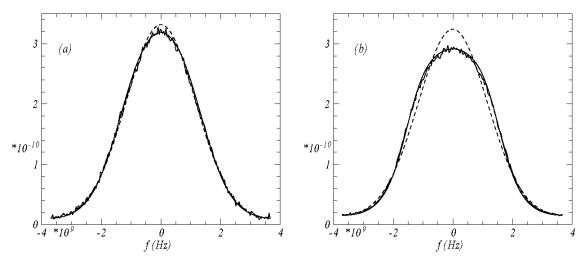
Figure 9-1: Spontaneous Rayleigh-Brillouin scattering on dry air, with the measured line shape compared to the Rayleigh line profile for (a) p = 0.3 bar and (b) p = 1 bar. The experiments, and the way in which they are compared to the model are explained below.
