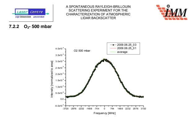
Figure 7-17: To compare different measurements, in which the intensity may vary, the intensity scale is normalized to area equal to one.
