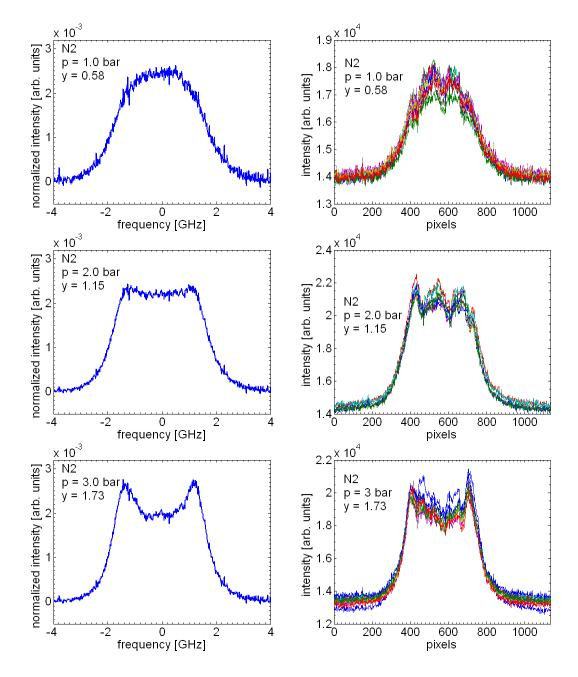
Figure 8-1: Experimental results on Coherent Rayleigh Brillouin scattering at 532 nm for various pressures in  $N_2$ . On the right raw data, on the left averaged data.
