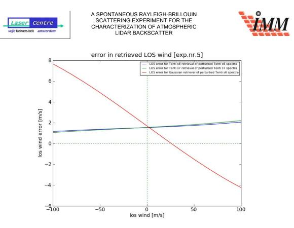
Figure 11-25: LOS wind error calculated from the residuals from experiment 5 (pressure 725 hPa).
