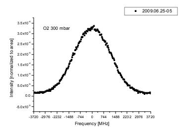
Figure 7-16: To compare different measurements, in which the intensity may vary, the intensity scale is normalized to area equal to one.
