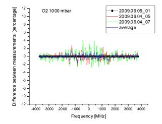
Figure 7-21: Residual plots of the difference between the measurements (and the average), in percentage of the amount of (normalized) signal.
