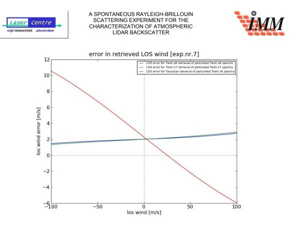
Figure 11-27: LOS wind error calculated from the residuals from experiment 7 (pressure 1040 hPa).
