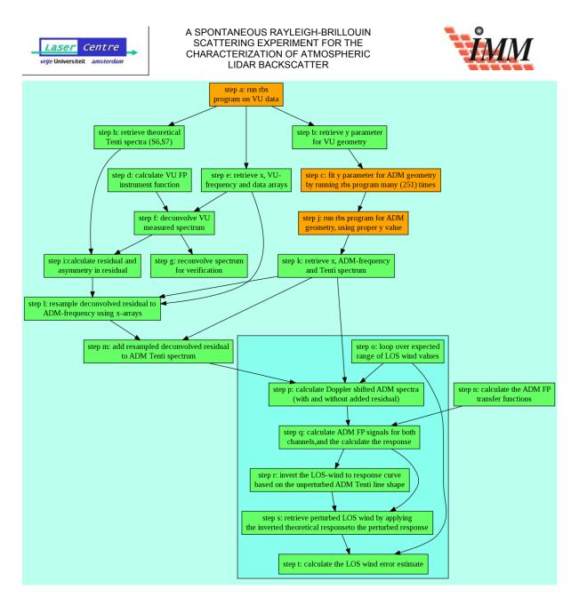
Figure 11-9: Flow-diagram of the steps needed to estimate the expected uncertainty in the LOS wind due to the uncertainty (residual) in the spectral shape.
