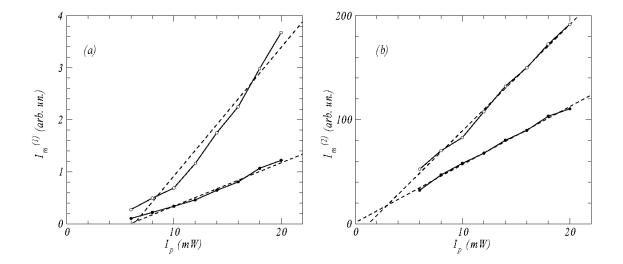
Figure 9-18: Coherent Rayleigh-Brillouin scattering signal versus pump power for N<sub>2</sub>. (a) Plotting as linear dependence (Eq. 9.22), (b) Plotting as quadratic dependence (Eq. 9.24). In both figures: dots correspond to p = 2 bar and open circles to p = 3 bar.
