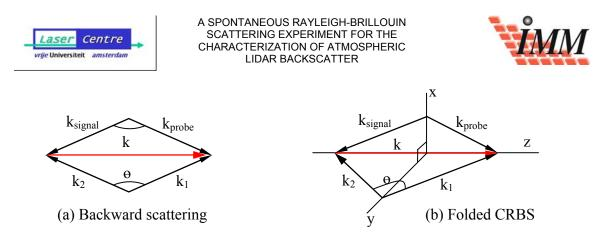
Figure 3-2: Phase matching schemes for coherent Rayleigh-Brillouin scattering.  $k_1$  and  $k_2$  are the pump beams' wave vectors. k is the wave vector of the induced density perturbation.
