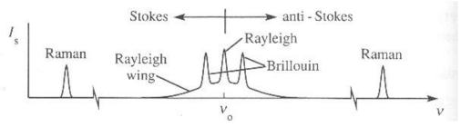
Figure 2-1: Spectrum of the Rayleigh scattered radiation, with incident radiation at frequency  $v_o$ .
