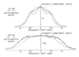
FIG. 2. The spectrum of light scattered from Xe and  $CO_2$  at an angle of 169.4° and pressures near one atmosphere. The curves are experiment (solid), Maxwell molecule theory (dotted), Krook model theory (dashed), and the hydrodynamic approximation (dash-dotted).
