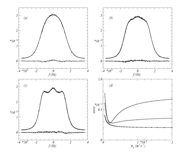
Figure 9-9: O<sub>2</sub> coherent Rayleigh-Brillouin scattering. (a) p = 1 bar,  $\eta_b = 2.021 \times 10^{-5}$  kg m<sup>-1</sup>s<sup>-1</sup> (the literature value); (b) p = 2 bar,  $\eta_b = 2.021 \times 10^{-5}$  kg m<sup>-1</sup>s<sup>-1</sup>; (c) p = 3 bar,  $\eta_b = 2.021 \times 10^{-5}$  kg m<sup>-1</sup>s<sup>-1</sup>, (d) Error as a function of  $\eta_b$ , dots, open circles and open squares, p = 1, 2, 3 bar, respectively.
