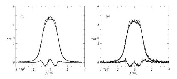
Figure 9-17: Krypton, p = 1 bar, comparison to the Marquez mixture model. (a) spontaneous Rayleigh-Brillouin scattering, (b) coherent Rayleigh-Brillouin scattering.
