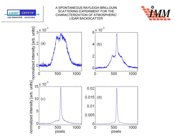
Figure 3-16: Spectral narrowing of the scattering signal for different displacements of pump1 beam and thereby different scattering angles  $\theta$  with respect to pump2 and probe beams. From figure (a) to (d) the scattering angle is increased by adjusting the mirror mount.
