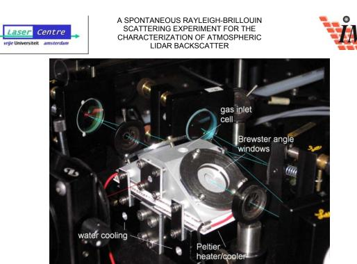
Figure 5-27: The cell mounted inside the enhancement cavity.
