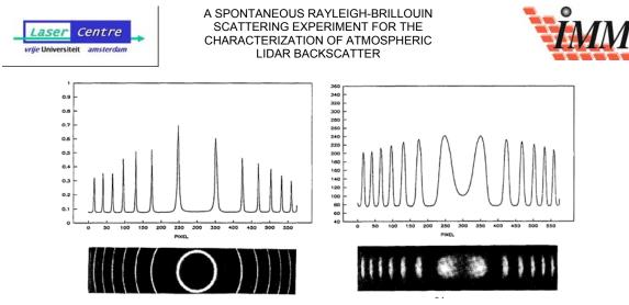
Figure 4-6: Results obtained by Lock et al. Left: the instrumental function of the etalon. Right: the RBS spectrum of  $N_2$  at room temperature.
