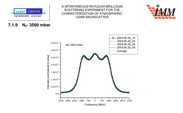
Figure 7-14: To compare different measurements, in which the intensity may vary, the intensity scale is normalized to area equal to one.
