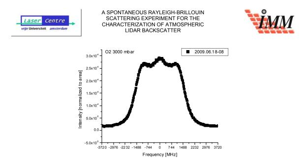
Figure 7-25: To compare different measurements, in which the intensity may vary, the intensity scale is normalized to area equal to one.
