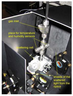
Figure 5-28: The cell mounted inside the enhancing cavity with the gas inlet to the cell.
