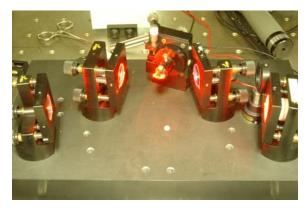
Figure 5-3: View on the frequency-doubling cavity in operation.
