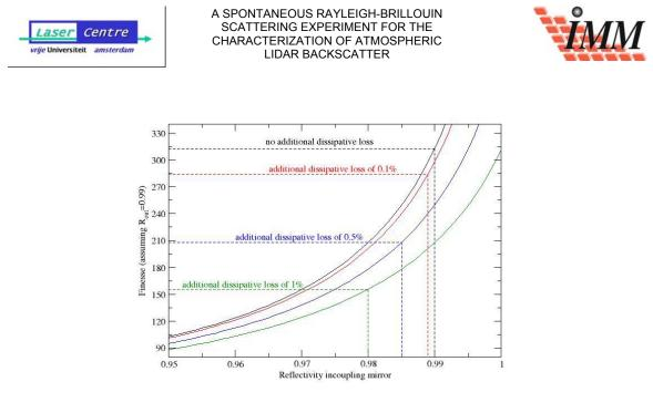
Figure 5-11: Variation of Finesse with the reflectivity of the input mirror for different amounts of dissipative losses. A perfect Gaussian beam is assumed, perfectly mode matched. The reflectivity of the input mirror that gives the maximum power in-coupling on each case is shown with a dotted line for each case.
