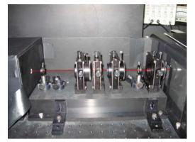
Figure 5-20: Light cleaning stage. The light goes from right to left, and its path is shown in red. The first holder contains the collecting lend L4, followed by a diaphragm (D2) and then by the set L5-S2-L6 of lens, pinhole and lens. The diaphragm D3 is the last components shown. The additional diaphragm  $D_2$  is placed to facilitate alignment, but it does not play any role in the signal collection.
