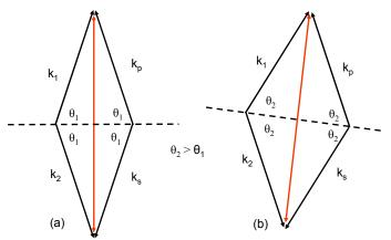
Figure 3-17: Phase matching scheme for (a) CRBS; (b) narrow-band scattering. Pump2 and the probe beam maintain the same direction, but pump1 and therefore also the scattering signal  $\theta$  change with respect to pump1 and probe beam.
