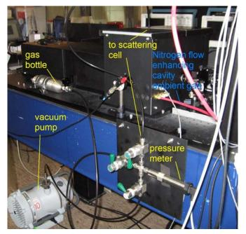
Figure 5-30: Mounted gas system for the SRBS experiments, the baratron shown is the APR 266.
