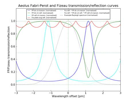
Figure 11-4: Simulated transmission and reflection on the active optical components used by the ADM-Aeolus detection system.
