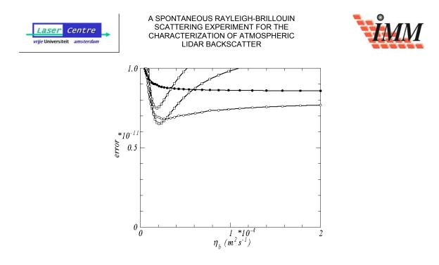
Figure 9-12:  $O_2$  coherent Rayleigh-Brillouin scattering. Same as Figure 9-11(d), but now the error is for the Tenti S7 model. For all pressures considered, the S7 model has significantly larger errors. There are two different experiments for p = 3 bar.
