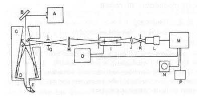
Figure 4-4: Experimental layout of the experiment by Sandoval and Armstrong [6]; scattered light at a forward angle of 15° is collected for signal detection of the Rayleigh-Brillouin spectrum. Note that both the input light to the Fabry-Perot interferometer and output light are filtered with sets of lenses and pinholes.
