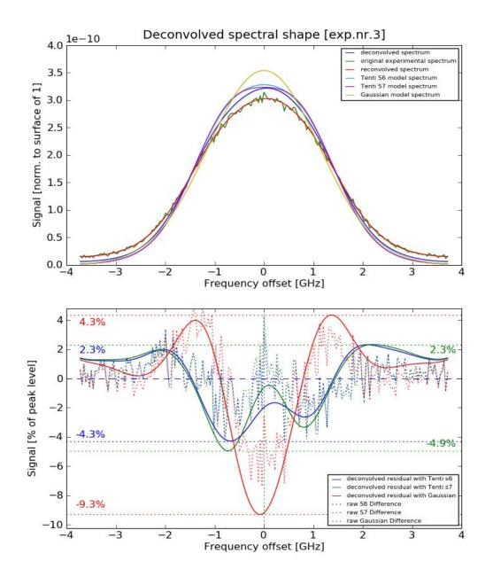
Figure 11-12: Deconvolution and residual calculation for experiment number 3 (pressure 504 hPa)
