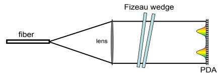
Figure 3-10: Fizeau spectrometer design. Light from a fiber is collimated by a lens and multiple beam interferences between two highly reflective mirrors in the Fizeau wedge causes an interference pattern to arise, which is simply recorded with a photodiode array (PDA).
