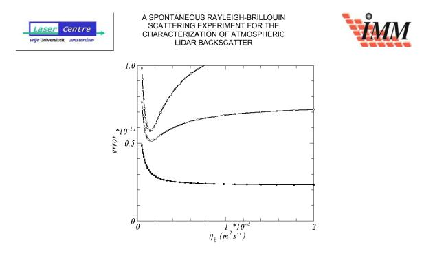
Figure 9-10:  $O_2$  spontaneous Rayleigh-Brillouin scattering. Same as Figure 9-9(d), but now the error is for the Tenti S7 model. For all pressures considered, the S7 model has significantly larger errors.
