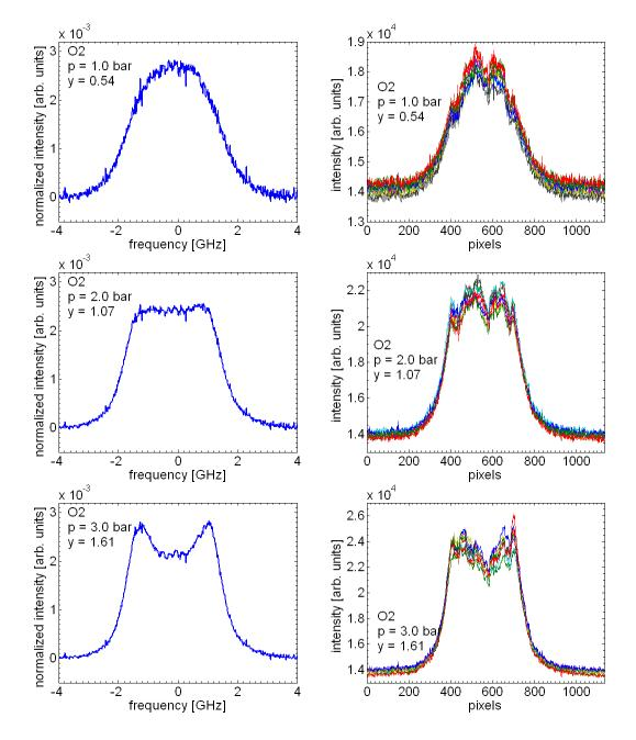
Figure 8-2: Experimental results on Coherent Rayleigh Brillouin scattering at 532 nm for various pressures in O<sub>2</sub>. On the right raw data, on the left averaged data.
