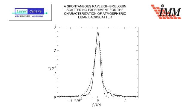
Figure 9-3: The response of the Fizeau interferometer. Full line: measured, dashed line: modeled by computing 128 repeated reflections of a plane monochromatic wave with  $\lambda = 532.2456$  nm,  $\theta_w = 17.05 \times 10^{-6}$  rad, and d = 14.9157 mm. Both response functions were used to compare models to experimental results.
