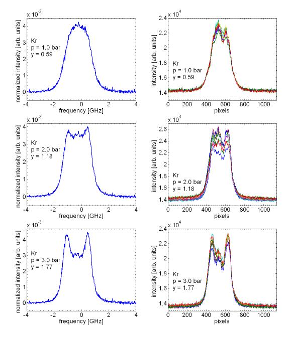
Figure 8-6: Experimental results on Coherent Rayleigh Brillouin scattering at 532 nm for various pressures in Kr. On the right raw data, on the left averaged data.
