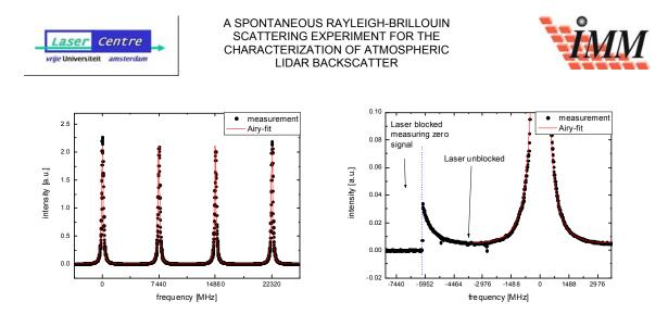
Figure 5-14: Airy fit of the transmitted function of the etalon, with the 4 modes in the etalon of approximately equal height. As it can be seen, the signal does not go to zero between the modes.
