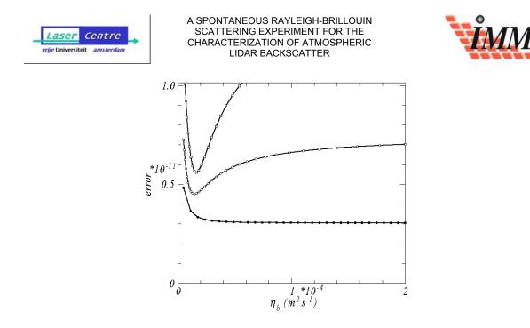
Figure 9-6: N<sub>2</sub> spontaneous Rayleigh-Brillouin scattering. Same as Figure 9-5(d), but now the error is for the Tenti S7 model. For pressures  $\geq$  2 bar, the S7 model has significantly larger errors.
