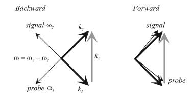
Figure 9-2: Arrangements of coherent Rayleigh-Brillouin scattering. The dipole forces  $a(k,\omega)$  are set up by the two pump beams with wave vectors  $k_1$  and  $k_2$ , and with the length of the scattering wave vector  $k = |k_s| = |k_1 - k_2|$ . The Rayleigh profile  $\omega = \omega_1 - \omega_2$  is picked from the broad spectral line shape of the pump beams. In the forward mode the beams are separated using polarizers.
