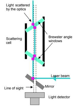
Figure 5-26: Schematic layout of the scattering cell mounted w.r.t. the enhancement cavity.
