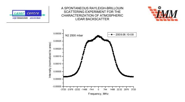
Figure 7-11: To compare different measurements, in which the intensity may vary, the intensity scale is normalized to area equal to one.
