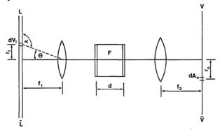
Fig. 1. Fabry–Perot interferometer used in the imaging mode. LL is the laser beam, F is the interferometer whose etalon plate spacing is d, and  $V\overline{V}$  is the CCD array. The scattering volume  $dV_i$  is imaged onto the pixel of area  $dA_0$  located at the coordinate  $\vec{r}_0$  on the array.
