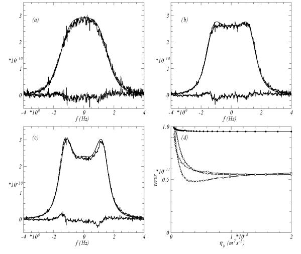
Figure 9-11: O<sub>2</sub> coherent Rayleigh-Brillouin scattering. (a) p = 1 bar},  $\eta_b = 2.021 \times 10^{-5}$  kg m<sup>-1</sup>s<sup>-1</sup>; (the literature value); (b) p = 2 bar},  $\eta_b = 2.021 \times 10^{-5}$  kg m<sup>-1</sup>s<sup>-1</sup>; (c) p = 3 bar,  $\eta_b = 2.021 \times 10^{-5}$  kg m<sup>-1</sup>s<sup>-1</sup>. (d) Error as a function of  $\eta_b$ , dots, open circles and open squares, p = 1, 2, 3 bar, respectively. There are two different experiments for p = 3 bar.
