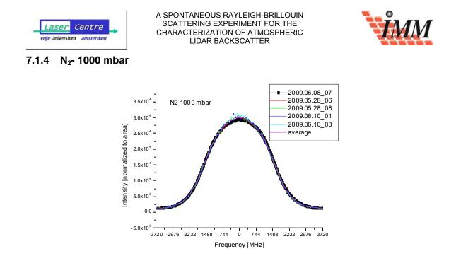
Figure 7-5: To compare different measurements, in which the intensity may vary, the intensity scale is normalized to area equal to one.
