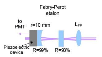
Figure 5-8: Design of the Fabry-Perot etalon.
