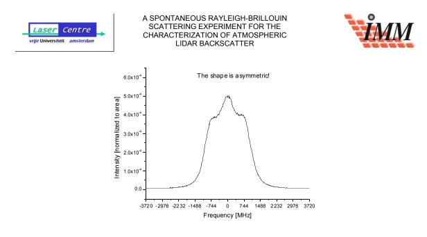
Figure 6-10: Measurement of Krypton at 3000 mbar. The obtained shape is asymmetric; the left shoulder is lower than the right shoulder of the Brillouin peaks.
