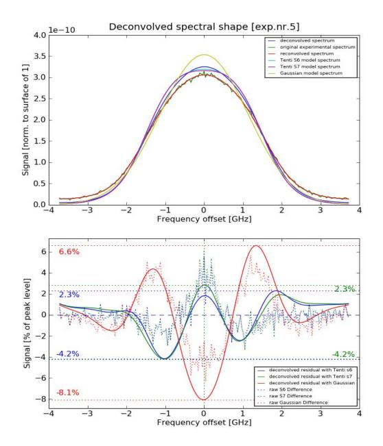
Figure 11-14: Deconvolution and residual calculation for experiment number 5 (pressure 725 hPa)
