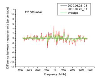
Figure 7-18: Residual plots of the difference between the measurements (and the average), in percentage of the amount of (normalized) signal.
