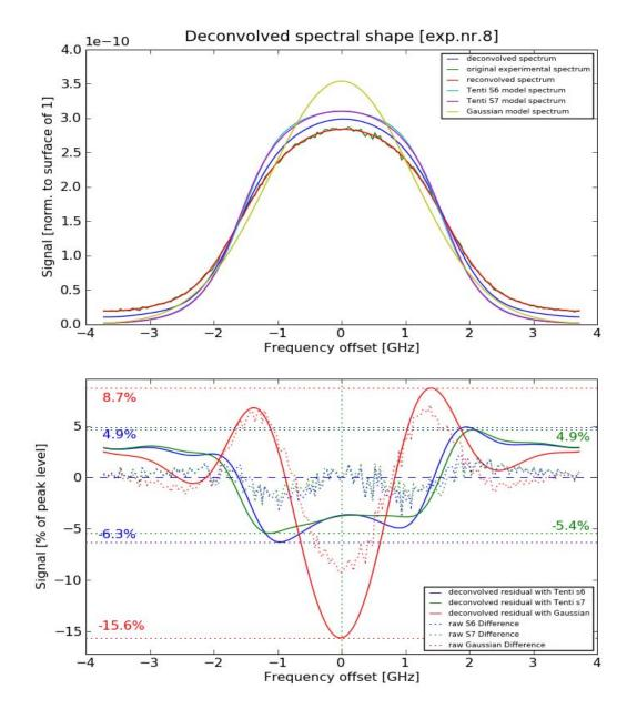
Figure 11-17: Deconvolution and residual calculation for experiment number 8 (pressure 1040 hPa)
