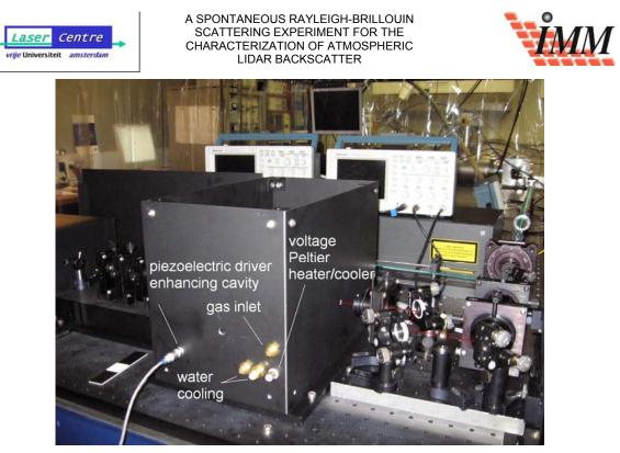
Figure 5-6: The enhancement cavity, together with the cell, is enclosed and flushed with  $N_2$ , to prevent external light, dust particles and contamination, and to have an atmosphere free of turbulence.
