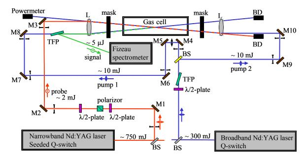
Figure 3-4: Two-dimensional CRBS setup. BS: beam splitter, TFP: thin film polarizer, M: mirror, BD: beam dump. Two pump beams originate from a broad-band Nd:YAG laser, while a probe beam is provided by an injection-seeded frequency-doubled Nd:YAG laser, and are focused by lenses in a gas cell. The scattered signal is spectrally analyzed by a Fizeau spectrometer.
