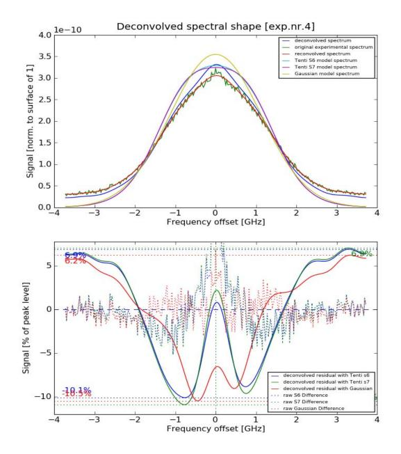
Figure 11-13: Deconvolution and residual calculation for experiment number 4 (pressure 500 hPa). Note that this experiment clearly suffered from some Mie contamination.
