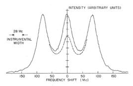
FIG. 1. The spectrum of light scattered from  $CO_2$  at an angle of 10.6° and a pressure of 770 mm of Hg, showing clearly resolved Brillouin components. At the maximum of one of the Brillouin peaks the signal produces about 300 photoelectrons/sec at the photocathode. The dashed curve indicates the subtraction of stray elastically scattered light.
