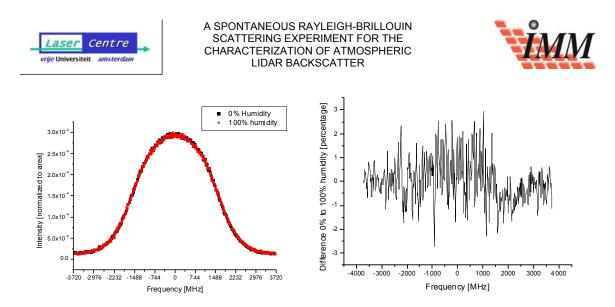
Figure 7-43: Measurements of 0% and 100% humidity alone for better comparison. The plot on the right is the difference between 0% humidity and 100% humidity, divided by the maximum value of the measurement with 0% humidity.
