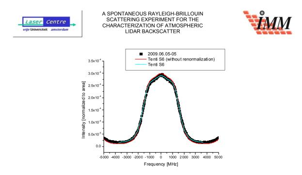
Figure 6-11: Measurement of  $O_2$  at 2000mbar. The model predicts a background level below the measured one; as a consequence, the normalization of the signal makes it appear higher. The curve in red is the model without re-normalization, the curve in blue is the same model, but the curve has been re-normalized to match the background of the measured signal.
