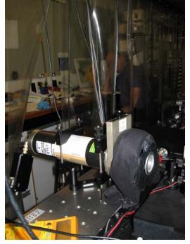
Figure 5-24: Picture of the PMT used in the experiment (Photonis XP2020 Q fast/high gain). In the background it can be seen the equipment used for data acquisition and computer.
