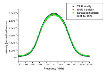
Figure 7-42: Measurements of air at 1000 mbar. The measurements were performed in the same conditions. The dry air measurement is similar to the measurements presented before. A drop of water was added into the cell and the measurement with "increasing humidity" was performed. Later a measurement with 100% humidity alone was done. The Tenti S6 model is plotted for comparison.
