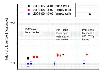
Figure 6-7: Average of the recorded signal on three different occasions. There are 3 different regimes where the signal is averaged: i) when the PMT is closed or the PMT is open and the laser is blocked, ii) when the PMT is open and the laser is circulating in the enhancing cavity, but the enhancing cavity is not locked, iii) when the PMT is open and the enhancing cavity is locked.
