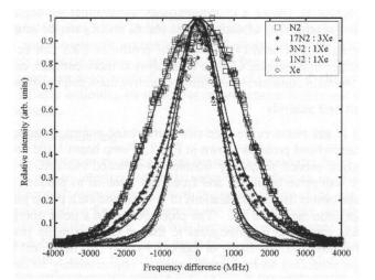
Figure 4-8: Rayleigh-Brillouin scattering spectrum of  $N_2$  diluted with Xenon gas at various relative gas compositions at total pressures of 100 mbar [25].
