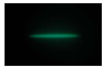
Figure 5-17: The length of the laser light in the image is around 2 mm (conditions of the photograph) and the diameter of the laser beam is ca 200  $\mu$ m. Note that there are no other sources of light, i.e. no scattered light from the optics or the scattering cell walls.
