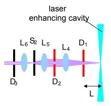
Figure 5-21: Stage for minimizing the opening angle for the RB-scattering.
