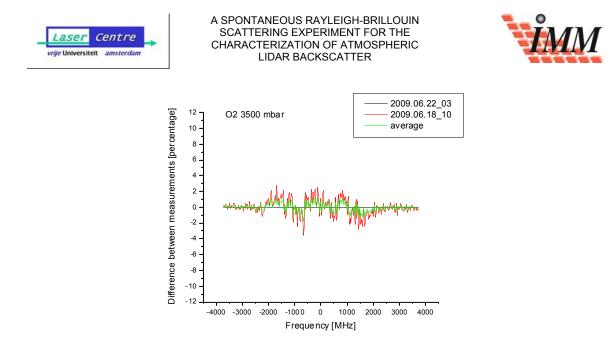
Figure 7-27: Residual plots of the difference between the measurements (and the average), in percentage of the amount of (normalized) signal.
