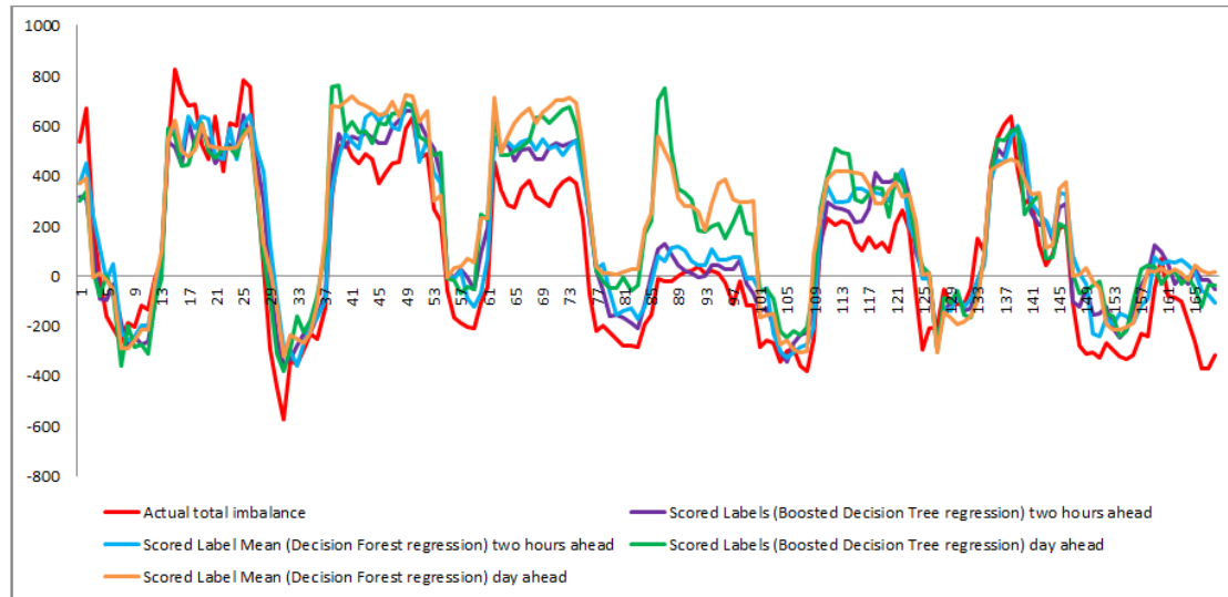
Figure 5.13. Forecast of the total imbalance for a week with the total imbalance from t-2 in the set of the predictors.
