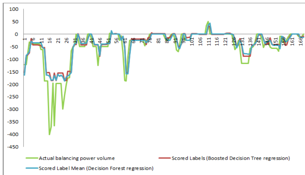
Figure 5.7. Forecast of the balancing power volume for a week with the balancing power volume from t-1 in the set of the predictors.
