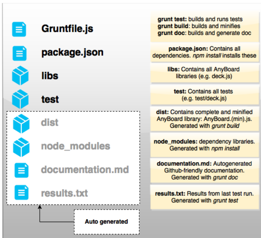
Figure A.2: Overview over the AnyBoard development files and folder structure.
