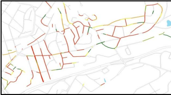
Figure 6 Visualization of pipes conditions with a GIS system (red = class 5, orange = class 4, yellow = class 3, dark green = class2, light green = class1)
