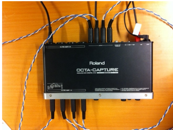
Figure 3.2: OCTA CAPTURE connected to four nodes, four inputs and four outputs.
