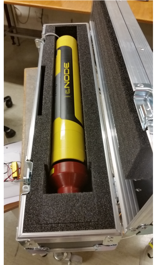
Figure 3.3: Transponder, cNODE, from Kongsberg Maritime during test. The transponder is connected to the sound card.
