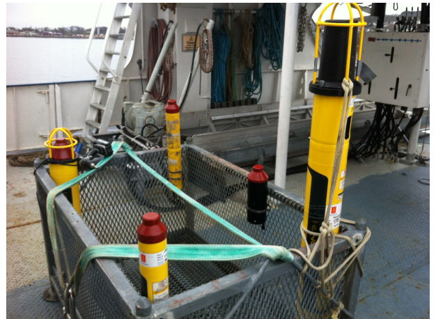
(b) Types of transponders, in this experiment only one is used
