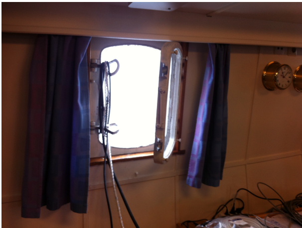
(a) A picture of the window from inside the boat. The hydrophone is placed out through a window, and connected to a computer via the sound card.
