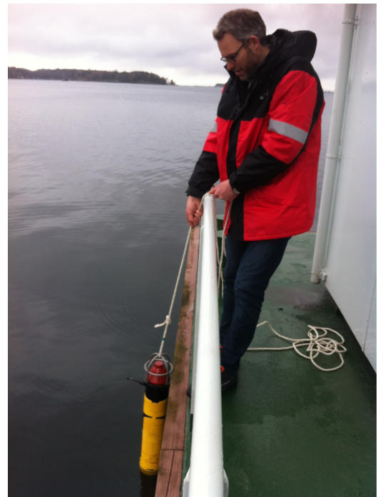
Figure 3.14: Thor Husøy deploying the transponder at the harbor.
