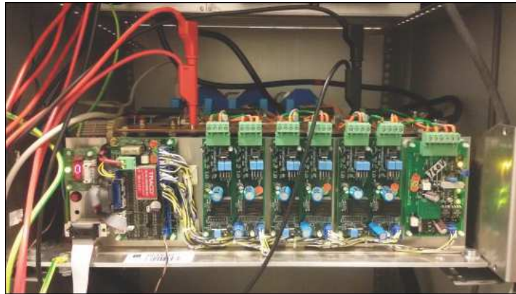
Figure 7.12: Driver circuit for inverter.
