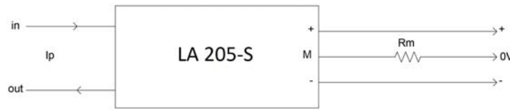
Figure 7.7: LEM current transducer connection block diagram.
