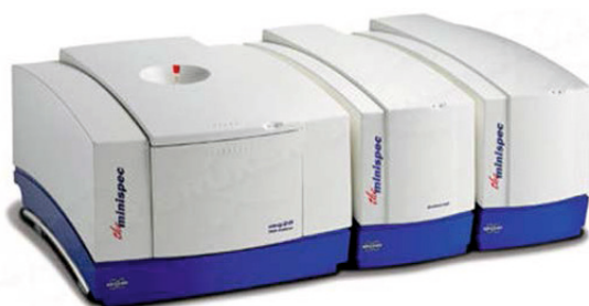
Figure 12. Picture of the low-field NMR bench top instrument.
