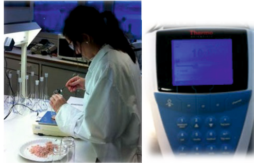
Figure 17. Sample preparation of cooked ham for measuring of sodium content with sodium selective electrode and a Dual Star™ pH/ISE Meter.
