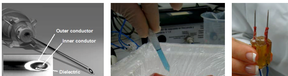
Figure 11 Sensor; needle electrode (left), arrowhead electrode (middle) and double electrode (right).
