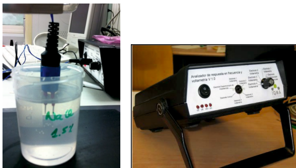
Figure 9 Impedance measurement in salt solution with a double electrode (left) and impedance Measurement equipment (right).
