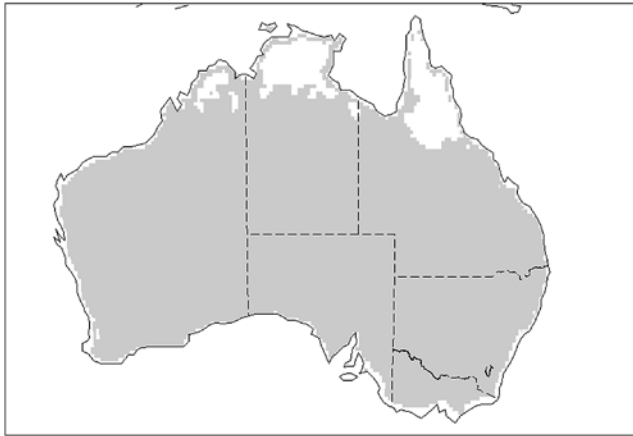
Figure 2. Map of Australia ( 10^{\circ}\text{S} – 40^{\circ}\text{S} , 110^{\circ}\text{E} – 160^{\circ}\text{E} ) showing the extent of missing SSM/I \theta retrievals for tropical northern Australia throughout the whole year. Most likely, data missing is due to the dense vegetation cover and high microwave frequency of SSM/I.
