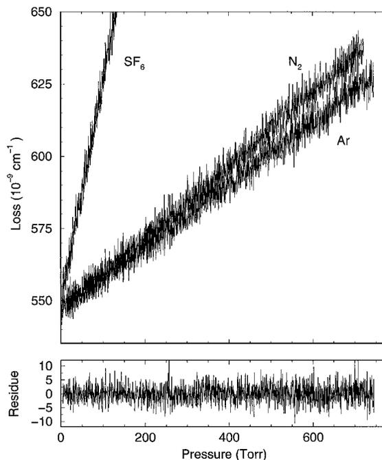
Fig. 1. Extinction owing to Ar,  $\text{N}_2$ , and  $\text{SF}_6$  as a function of pressure measured in the CRD setup. The bottom panel shows the residue of an unweighted linear regression of the Ar extinction curve (rms,  $3 \times 10^{-9} \text{ cm}^{-1}$ ; mean,  $4 \times 10^{-13} \text{ cm}^{-1}$ ).
