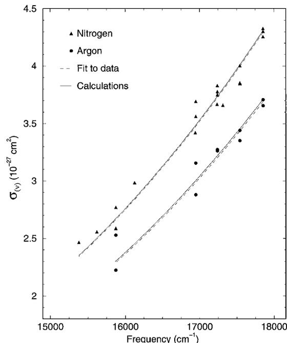
Fig. 2. Experimentally determined Rayleigh scattering cross sections for Ar and  $\text{N}_2$  compared with calculations.
