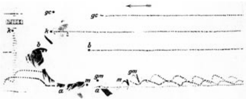
Figure 2 — Excerpt from a crescendo negative (#1064). One can see the scale plank with cm marks on the left; the right part of the Figure shows the last fragment of the crescendo kymocyclogram. The frequency of the recording is 60 strikes per second. For abbreviations, see the text.
